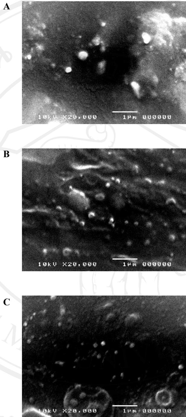
**Figure 21** SEM micrographs of TDE loaded SLN incorporated in nanocream at 0.25% (A), 0.50% (B) and 1.25% w/w (C)
