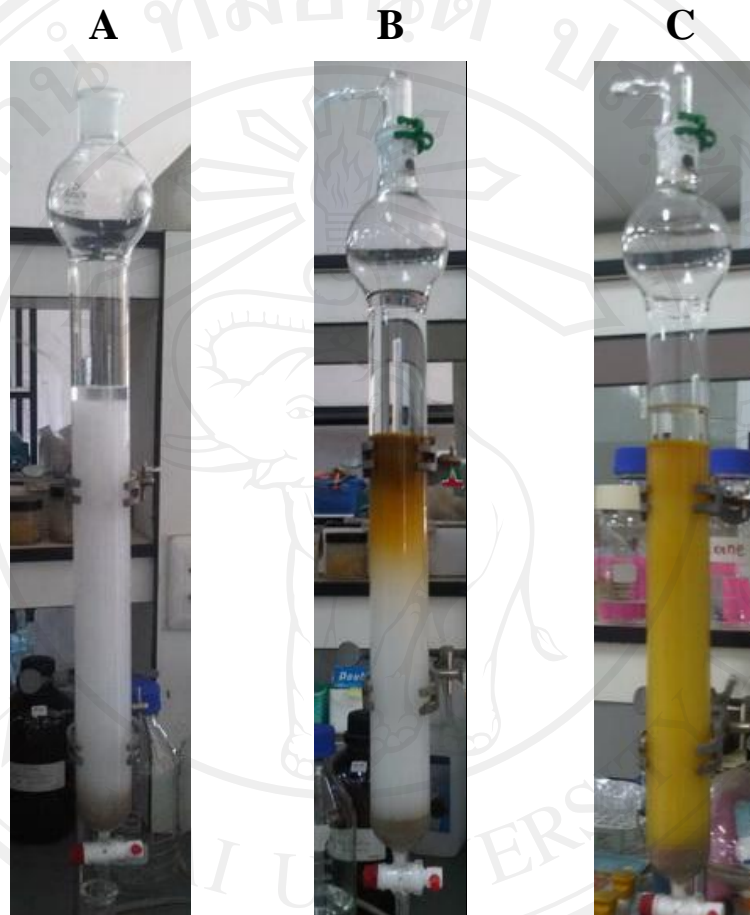
Figure 5 Column chromatography (50 mm diameter, 50 cm height) packed with silica gel (A), loading with crude extract of the T. laurifolia leaves dissolved in 95% ethanol (B) and the fractions (500 mL) were eluted by different ratio of ethyl acetate and methanol (C). The fractionated process took about six hours per one experiment.
