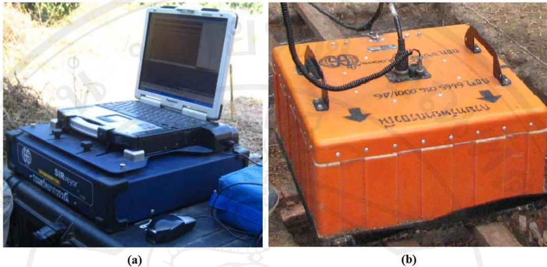
Figure 1.1. (a) GSSI SIR-20 GPR system with (b) 200 MHz antenna.
