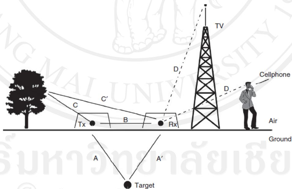
Figure 2.5. A ground penetrating radar (GPR) system emits and detects radio wave signals. There are many possible signals and paths and the objective is to maximize the target response and minimize others. (From Harry, 2009).
