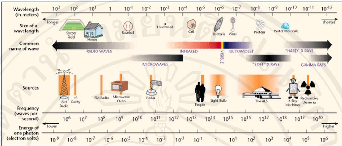
Figure 2.2. Electromagnetic wave spectrums. Wavelength, frequency and energy per photon are represented in top, middle and bottom scales, respectively. (From MicroWorlds, 2012).
