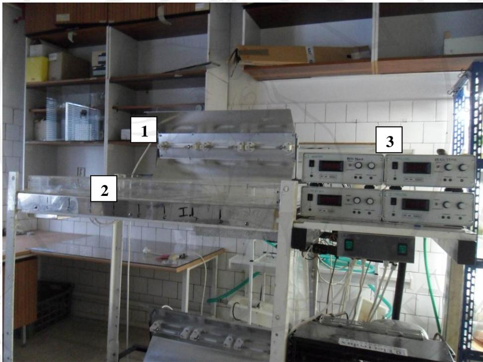
**Figure 7** The crossed gradients of light and temperature unit (Kviderova and Lukavsky, 2001). (1) = light irradiance sources (Osram Dulux L55W/12-950, Italy); (2) = the settle unit; (3) = cooling and heating control unit.
