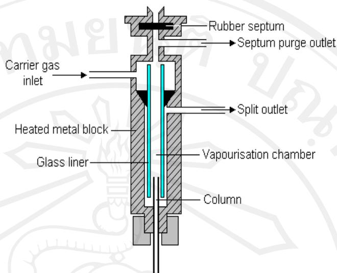
**Figure 1.20** Schematic diagram of a split/splitless injection port
