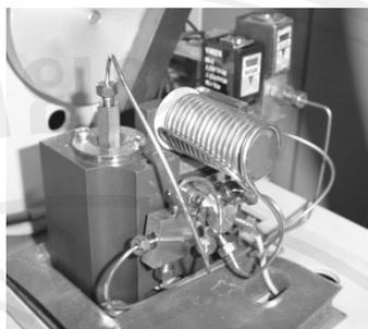
**Figure 1.16** Sample loop of headspace autosampler
