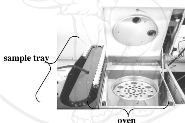
**Figure 1.15** Oven and sample tray of headspace autosampler
