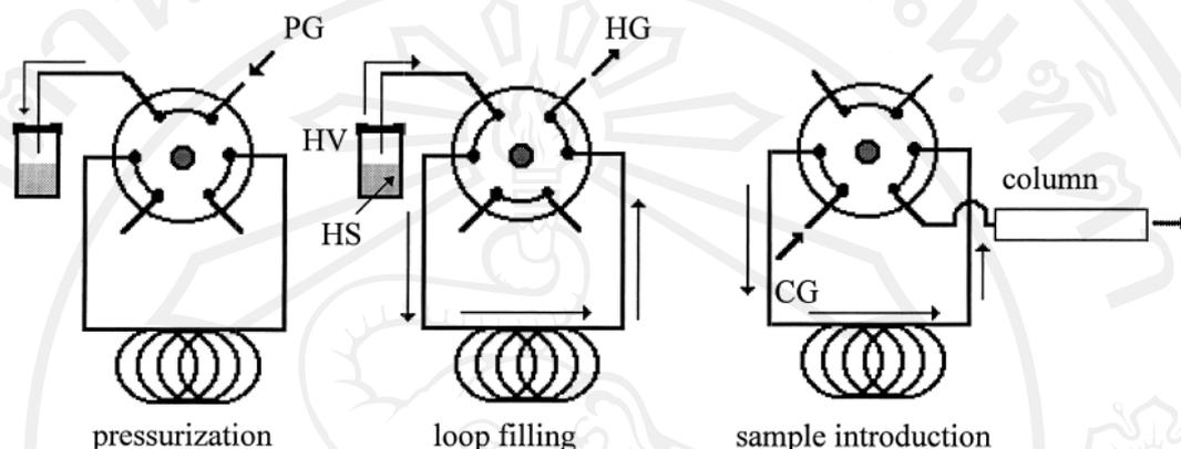
**Figure 1.18** Schematic of the ‘pressure/loop’ headspace sampling system. PG = Pressurization gas, HV = headspace vial, HS = headspace sample, CG = carrier gas
