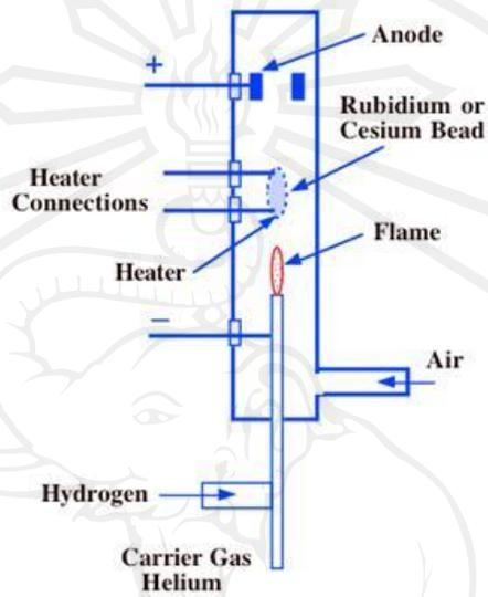
**Figure 1.21** A diagram of NPD detector<sup>54</sup>
