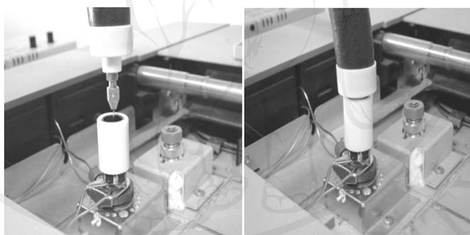
**Figure 1.17** Transfer line of headspace autosampler
