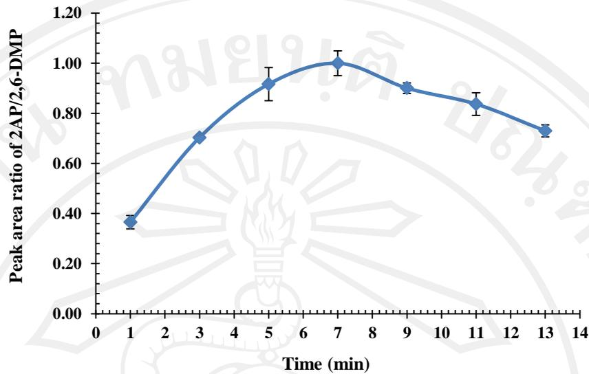
**Figure 3.9** Effect of equilibration times on peak area ratio of 2AP/2,6-DMP obtained at oven temperature at 110 °C.
