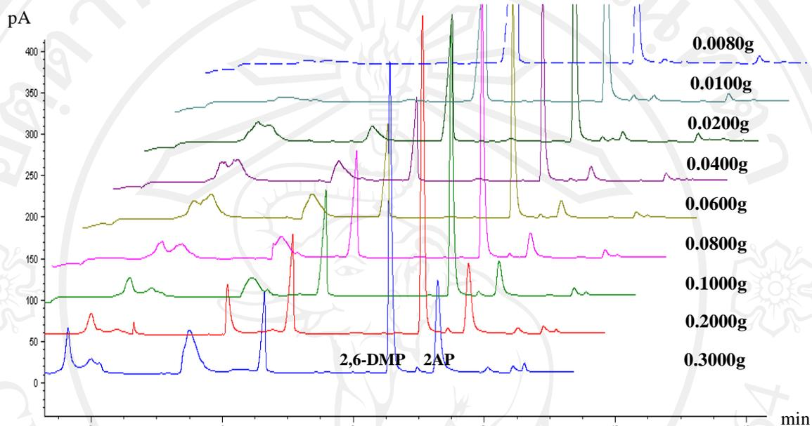
**Figure 3.21** SHS-GC/NPD chromatograms obtained by varying the amounts of KDML105 rice leaf sample at 0.3, 0.2, 0.1, 0.08, 0.06, 0.04, 0.02, 0.01 and 0.008 g.
