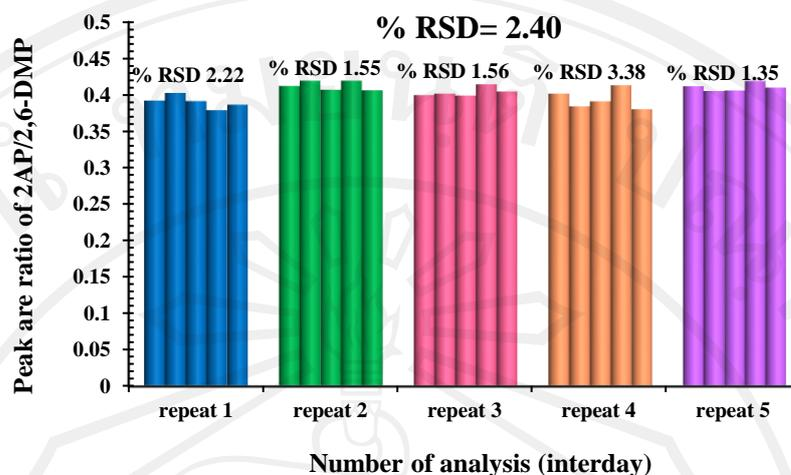
**Figure 3.23** Peak area ratios of 2AP/2,6-DMP in KDML105 rice leaves obtained by 5 replications of SHS-GC/NPD analysis within 5 days.
