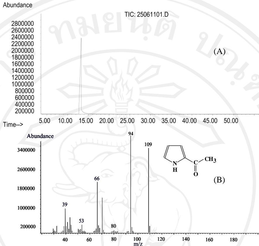
**Figure 3.1** GC-MS chromatogram (A) and mass spectrum (B) of the reactant, 2-acetylpyrrole.
