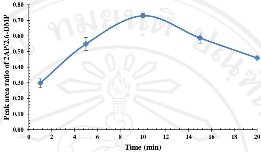
**Figure 3.8** Effect of equilibration times on peak area ratio of 2AP/2,6-DMP obtained at oven temperature at 100 °C.
