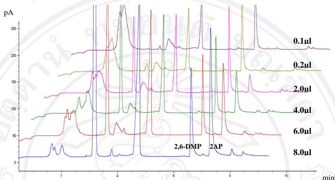
**Figure 3.20** SHS-GC/NPD chromatograms obtained by adding 1000 ppm of 2AP standard solution into headspace vial containing 0.2000 g of the non-aromatic rice (cv. Supanburi 2) at 8.0, 6.0, 4.0, 2.0, 0.2 and 0.1  $\mu\text{l}$ .
