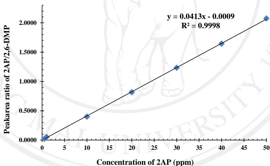
**Figure 3.19** Calibration graph of 2AP obtained by using SHS-GC/NPD.
