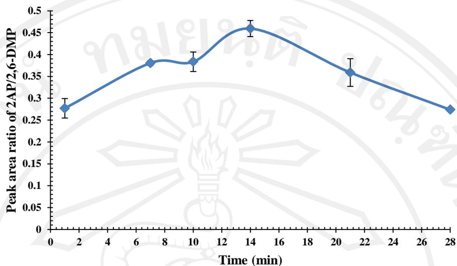
**Figure 3.7** Effect of equilibration times on peak area ratio of 2AP/2,6-DMP obtained at oven temperature at 90 °C.
