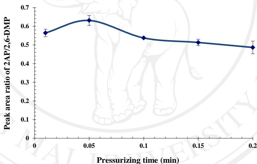
**Figure 3.13** Effect of pressurization time on peak area ratio of 2AP/2,6-DMP.
