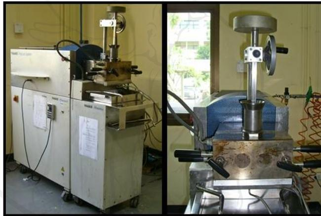
Figure 2.11 The HAAKE PolyLab internal mixer used in melt-mixing method.
