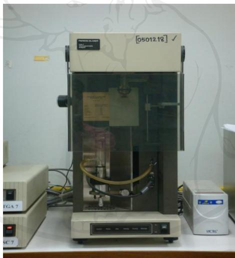
Figure 2.16 The Perkin-Elmer (TGA7) thermogravimetric analyzer used for thermal degradation.
