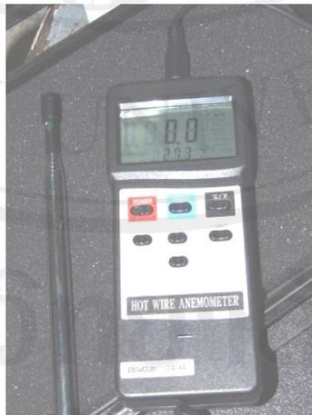
Figure 4.5 Hot wire anemometers for measuring air speed.
