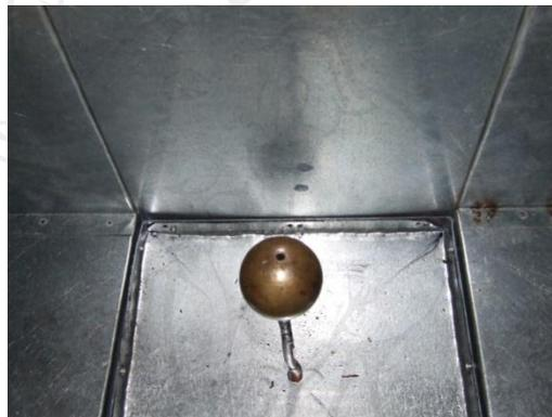
Figure 4.4 Fixing the sphere with the oil feeding tube.
