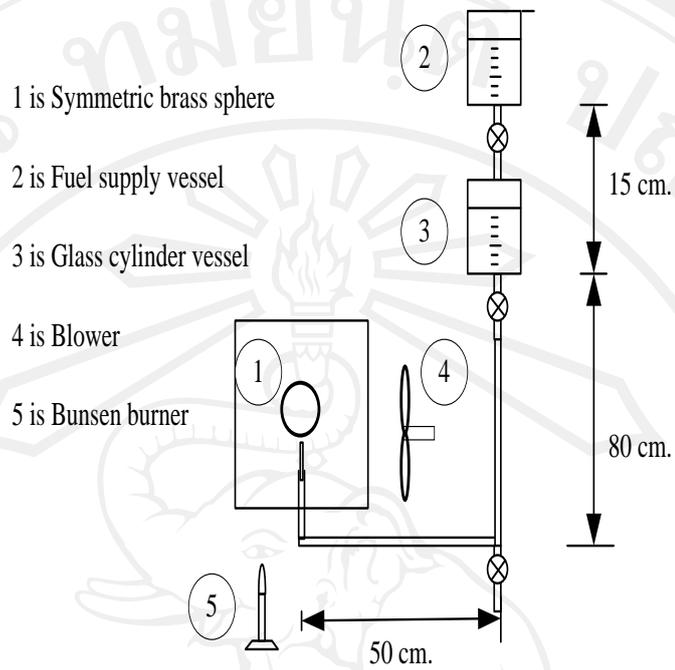
Figure 4.1 Experimental setup for testing single droplet combustion.
