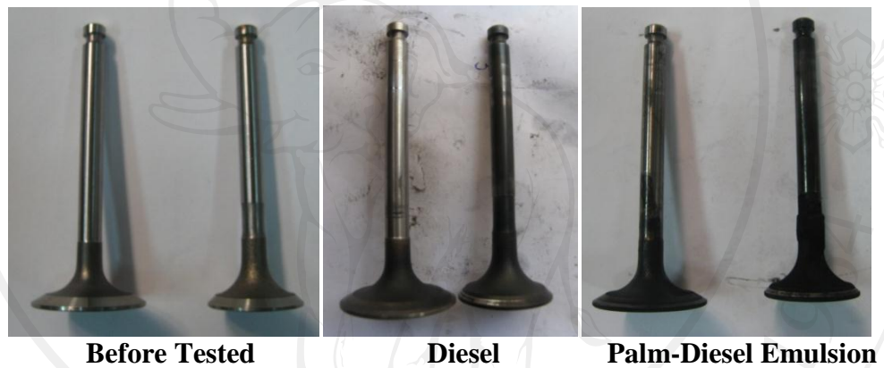
Figure 5.14 Wear at the intake valve and exhaust valve for the fuel oil and the emulsified Diesel/CPO/water of 90/5/5 after 200 h operation.
