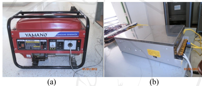
Figure 3.12 (a) Gasoline Generator with output is 220 VAC and (b) AC/DC inverter with output is 24 VDC
