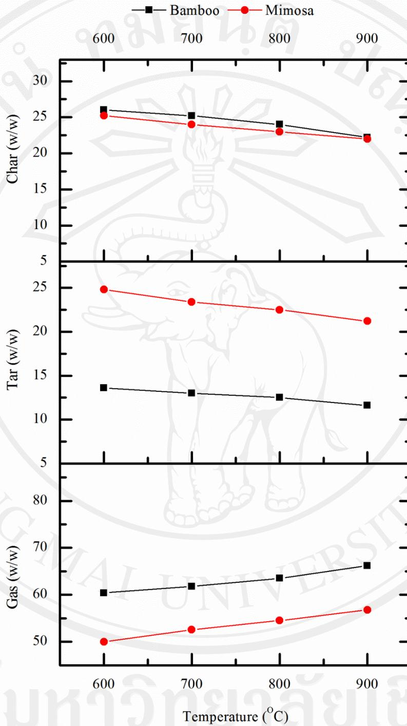
Figure 5.16 Effect of temperature on product yields in a fixed bed reactor
