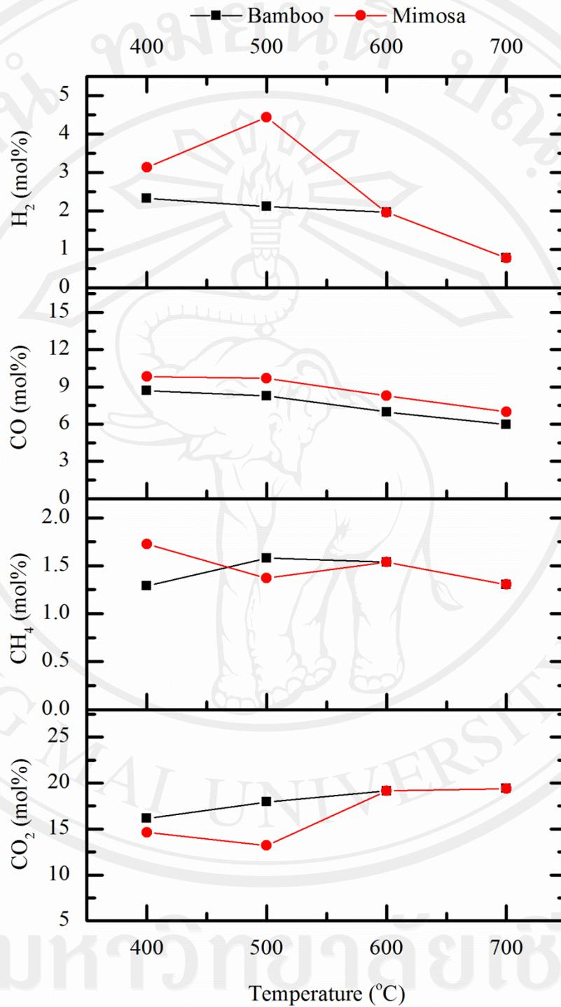
Figure 5.29 Effect of temperature on gas composition in a fluidized bed reactor
