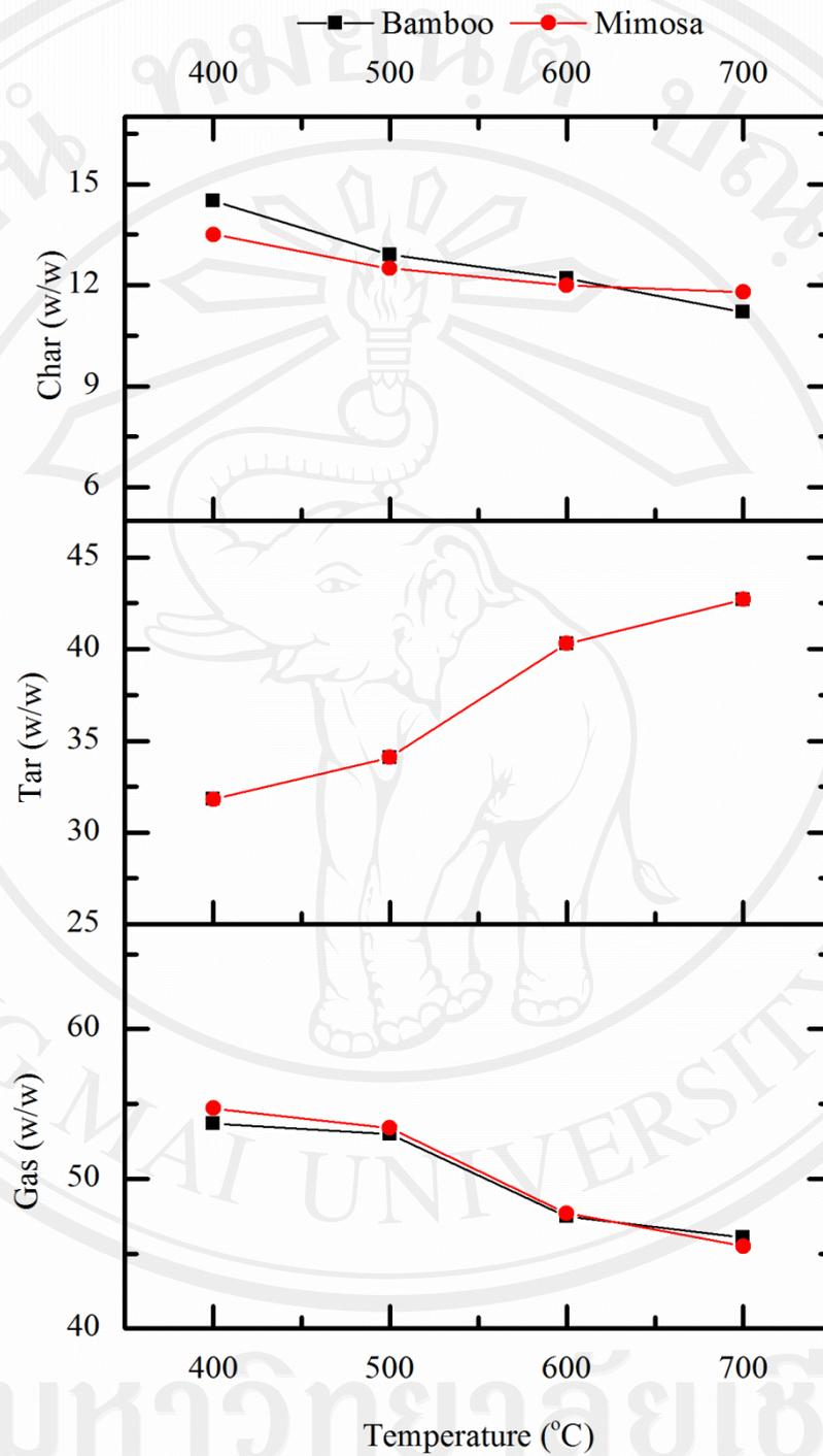
Figure 5.28 Effect of temperature on product yields in a fluidized bed reactor
