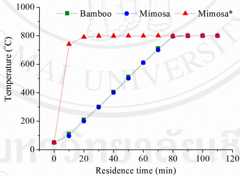
Figure 5.23 Temperature profile of biomass in fixed bed during gasification process in a fixed bed reactor
