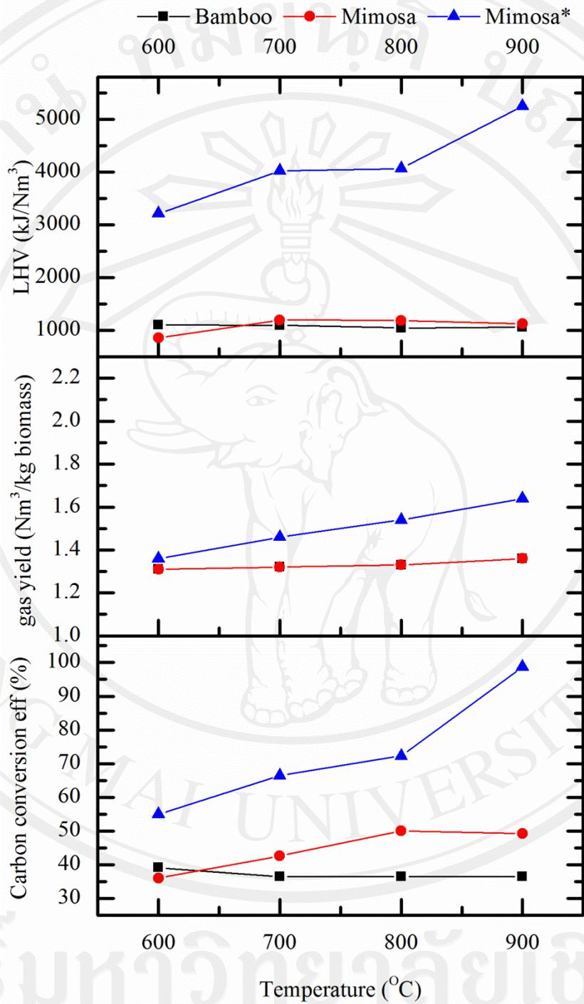
Figure 5.20 Effect of temperature on gas heating value, gas yields and carbon conversion efficiency in a fixed bed reactor.
