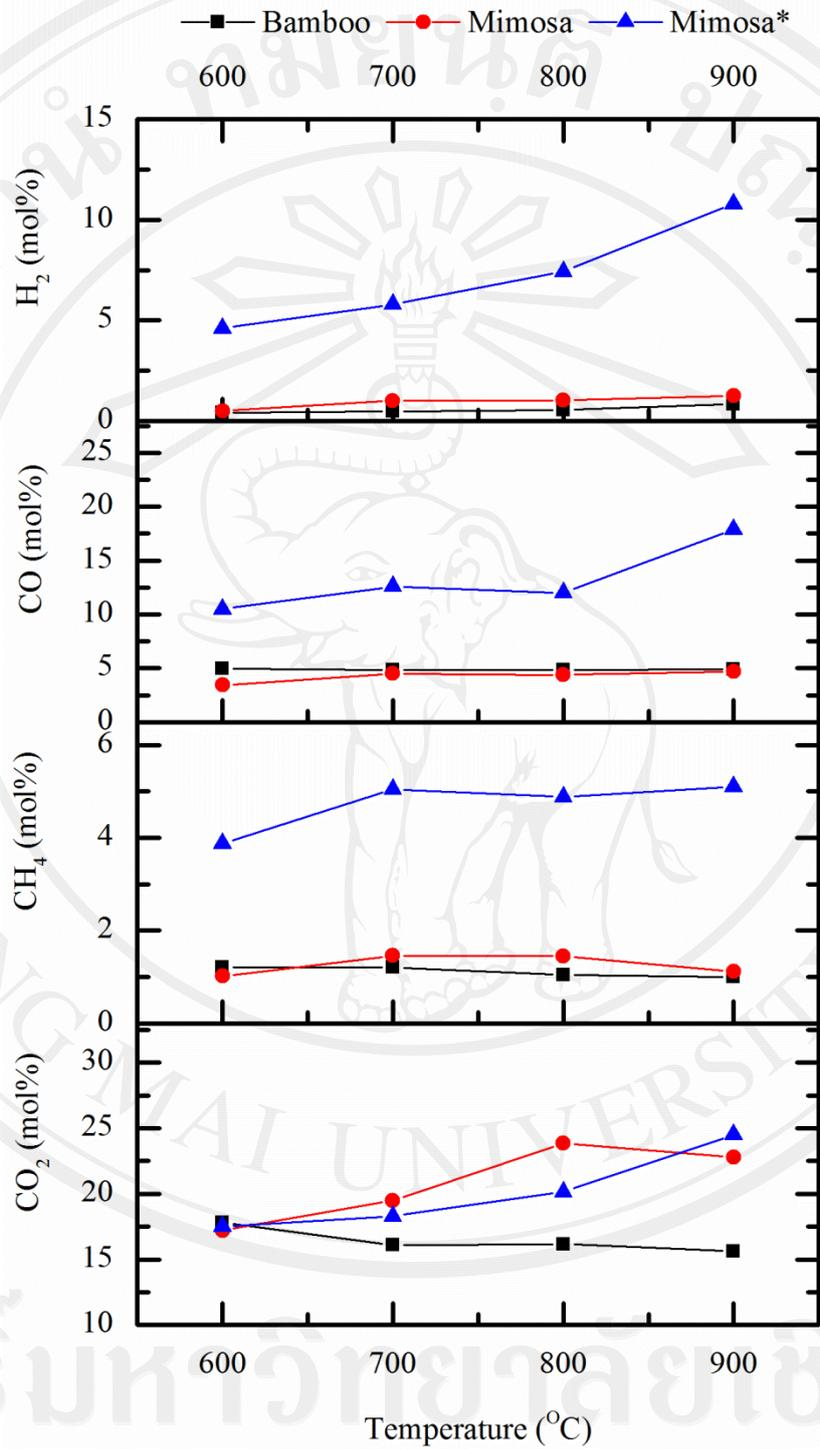
Figure 5.18 Effect of temperature on gas yield in a fixed bed reactor
