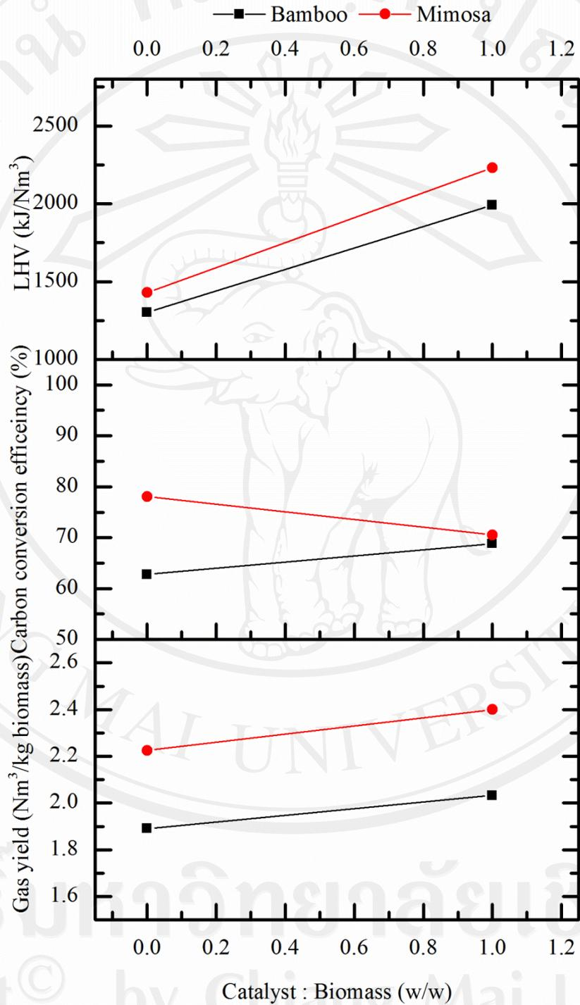
Figure 5.35 Effect of catalyst to biomass ratio on gas heating value , gas yields and carbon conversion efficiency in a fluidized bed reactor
