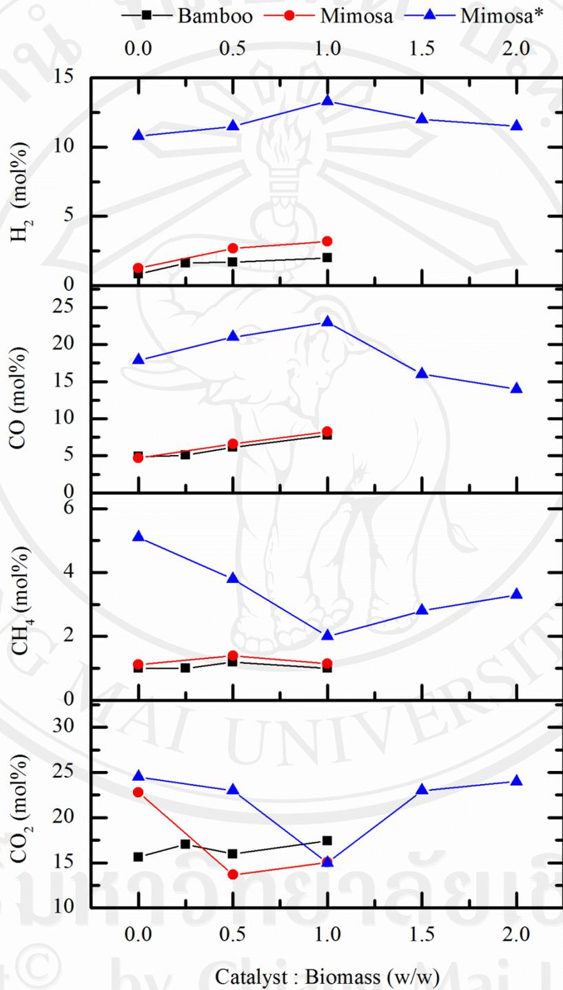
Figure 5.25 Effect of catalyst to biomass ratio on gas yields in a fixed bed reactor
