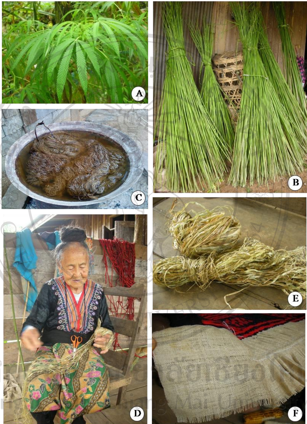
Figure 83. Hmong traditional way to make clothes from hemp A: Hemp ( Cannabis sativa ) B: Hemp stems used as source of hemp fiber C: Hemp fiber was boiled to make it soft D: Hmong woman is working with hemp fiber E: Hemp fiber F: Fabric made of hemp fiber
