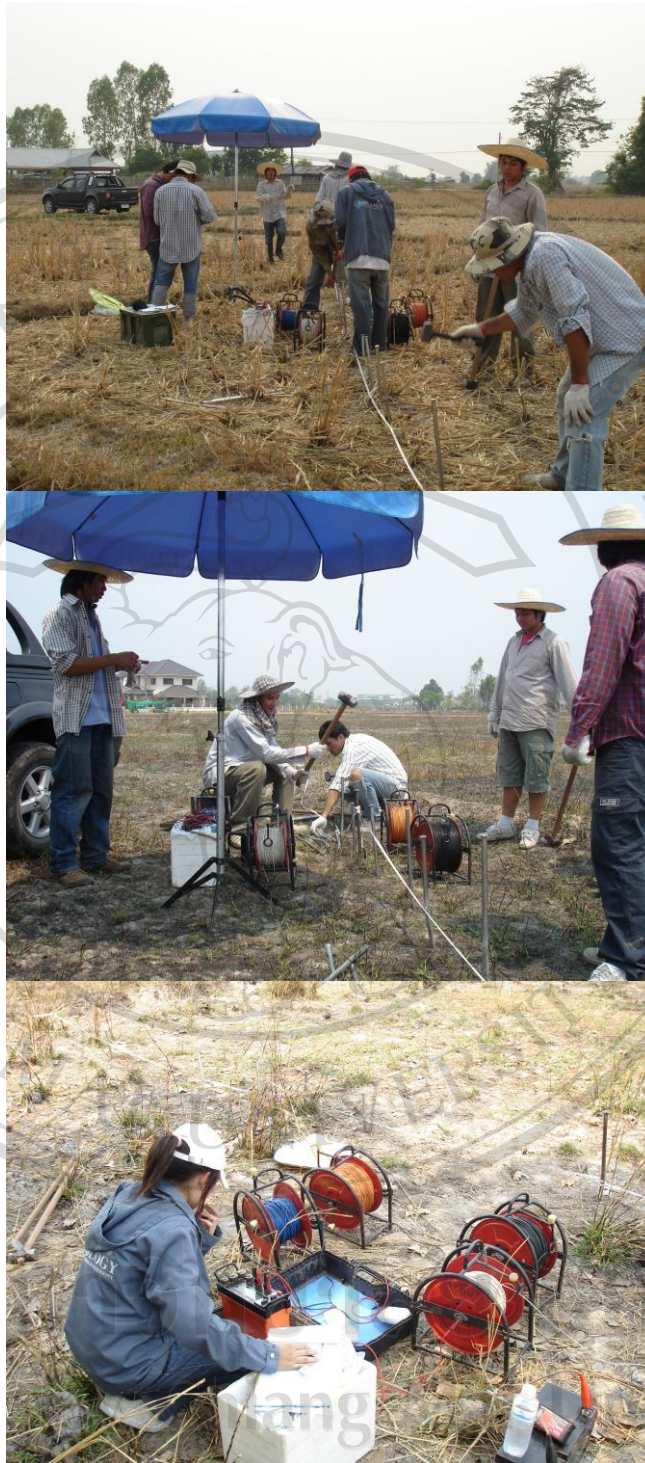
Figure 3.14 Electrical resistivity field surveys.
