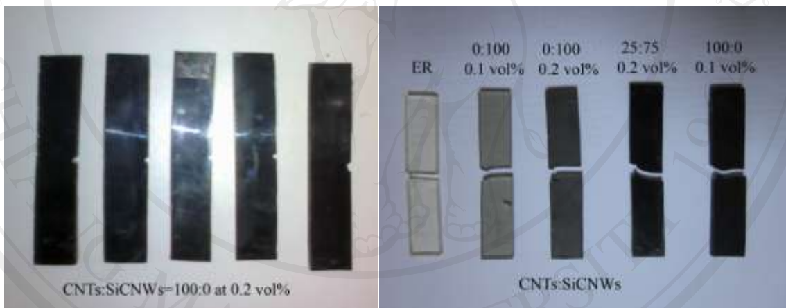
Figure 4.20 Before (CNTs:SiC ratio and after impact test of CNTs, SiCNWs and epoxy matrix samples
