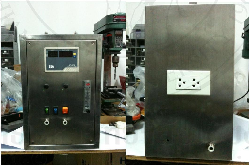
**Figure 2.12** Temperature and humidity controller of exposure chamber
