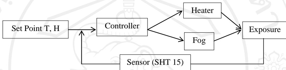
**Figure 2.11** Schematic diagram of the control system of temperature and humidity in chamber
