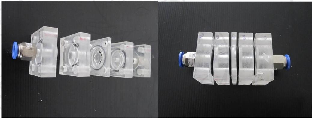
**Figure 2.4** Construction of the impactor for separation of PM10
