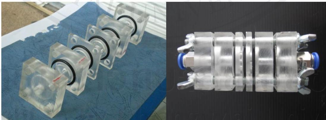
**Figure 2.5** Construction of the impactor for separation of PM2.5
