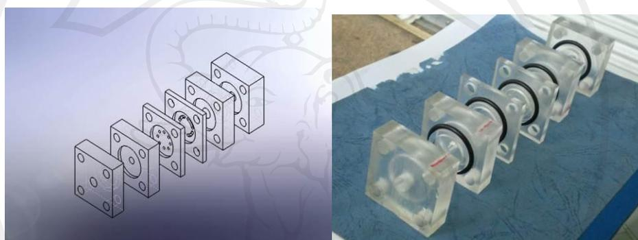
**Figure 2.3** Three-dimensional images of air impactor filter and prototype
