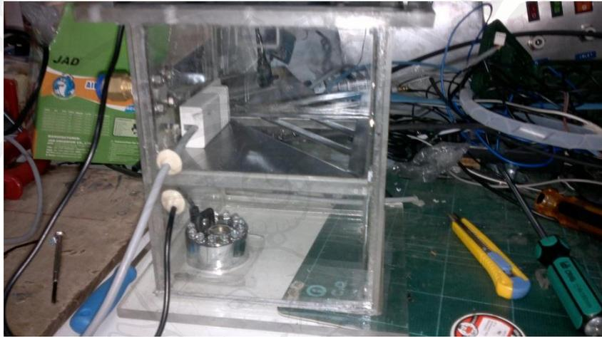
**Figure 2.6** The exposure chamber consists of three parts; temperature and humidity sensors, heater and moisture system.
