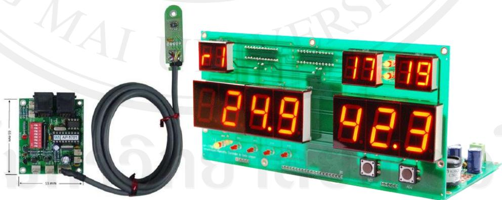
**Figure 2.10** Temperature and Humidity controller
