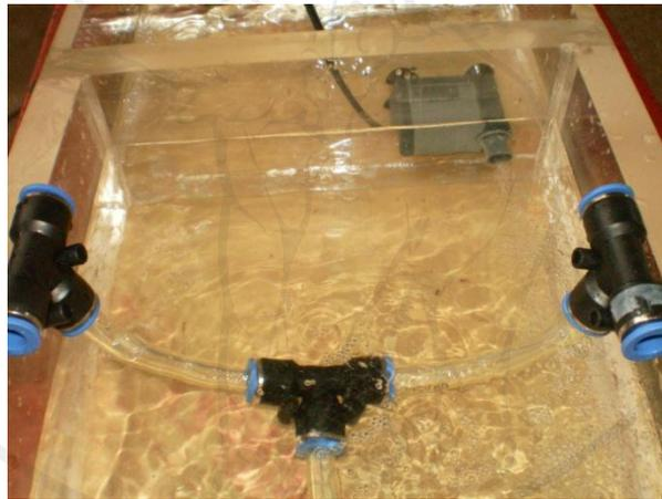
**Figure 3.6** The temperature was controlled by water bath.
