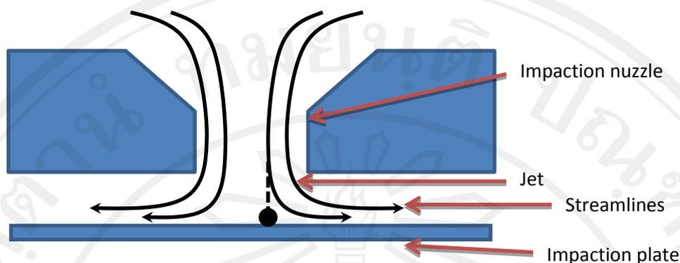
**Figure 3.9** Cross-sectional view of an impactor.
