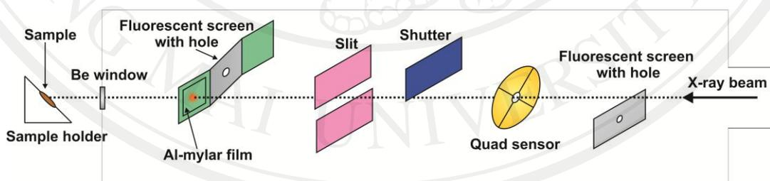
Figure 3.5: The beam diagnostics components.
