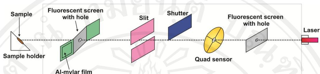
Figure 3.6: The alignment using laser beam.
