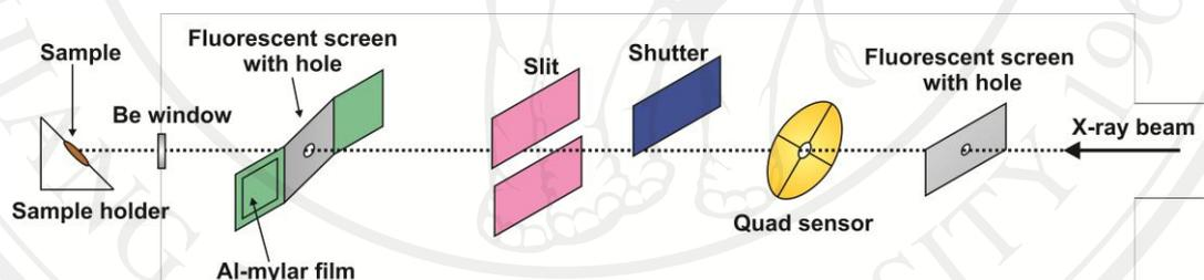
Figure 3.7: The alignment using x-ray beam.
