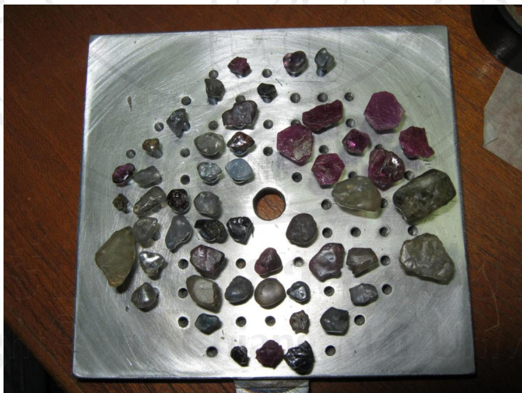
Figure 3.10. The sample holder used for \text{Ar}^+ and \text{N}_2^+ ion beam irradiations.
