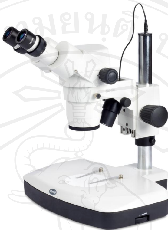
Figure 3.4. Motic SMZ-168 Series of stereomicroscopes (Motic., n.d.) used in this study.
