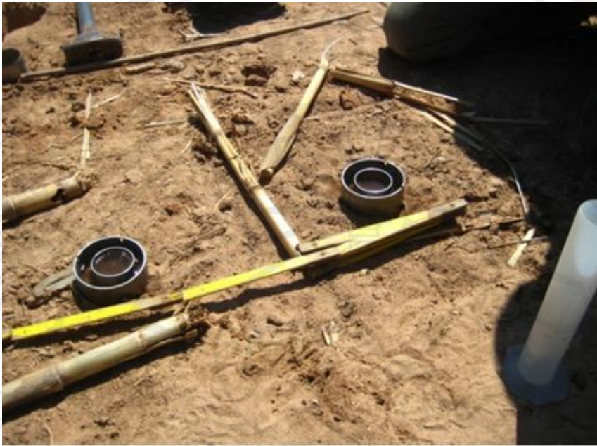
Figure 15: Double ring infiltrometer inside and outside CF station
