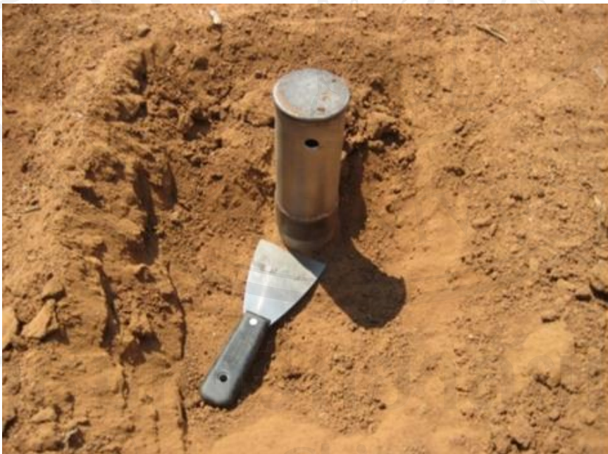
Figure 16: Bulk density sampling at 0-15 cm.
