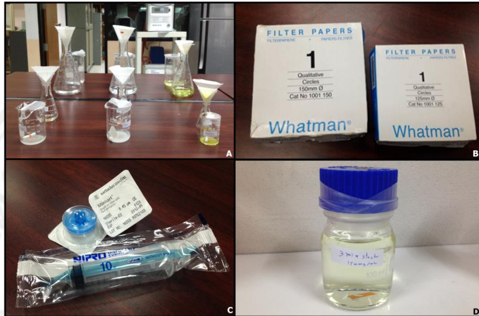
Figure 22: Preparation of 3Mix stock solution. The dissolved single antibiotic was sterilized by passing through 2 \mu\text{m} filtering papers (A, B) and 0.2 \mu\text{m} microfilters (C). Then a known concentration of 3Mix solution was prepared by mixing each drug at equal volume to a final concentration of 150.00 \mu\text{g}/\text{mL} 3Mix stock solution (D).
