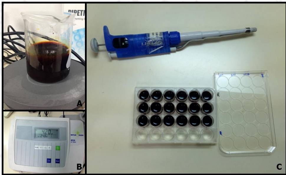
Figure 24: The alizarin red-S staining method for mineralization assay. The alizarin red-S solution was prepared at pH 4.2 (A,B). The specimens were rinsed with that solution for 5 minutes (C) with gentle rocking.
