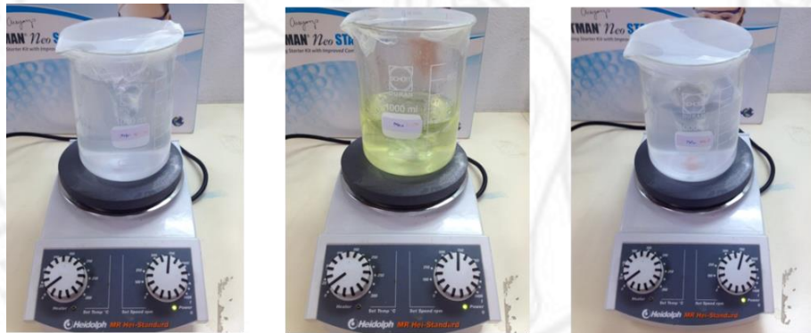
Figure 21: Preparation of 3Mix in water. Each antibiotic powder was dissolved in measured DI water and unified using magnetic stirrer in a separated beaker.
