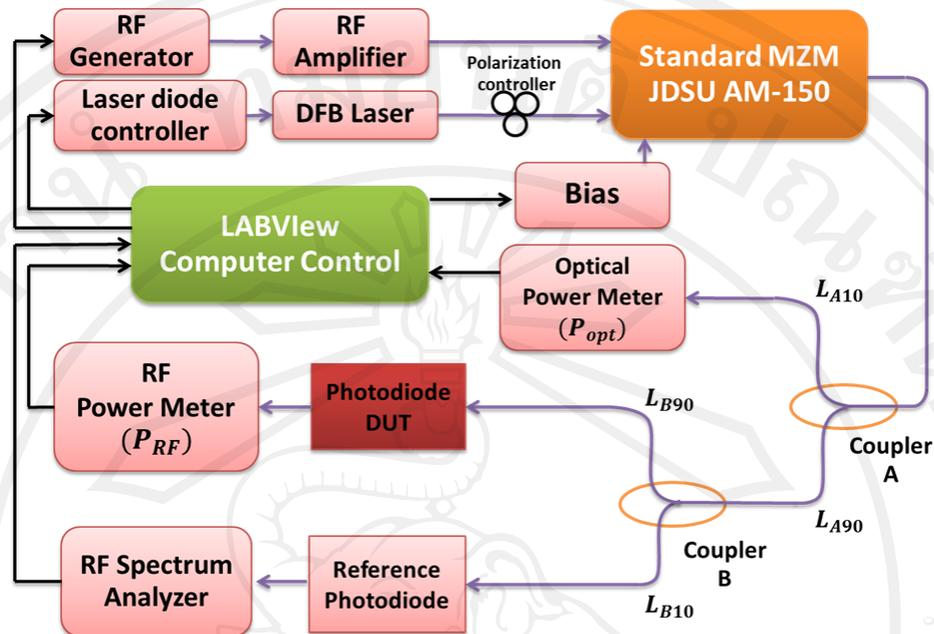
Figure 3.1 PD frequency response measurements system
