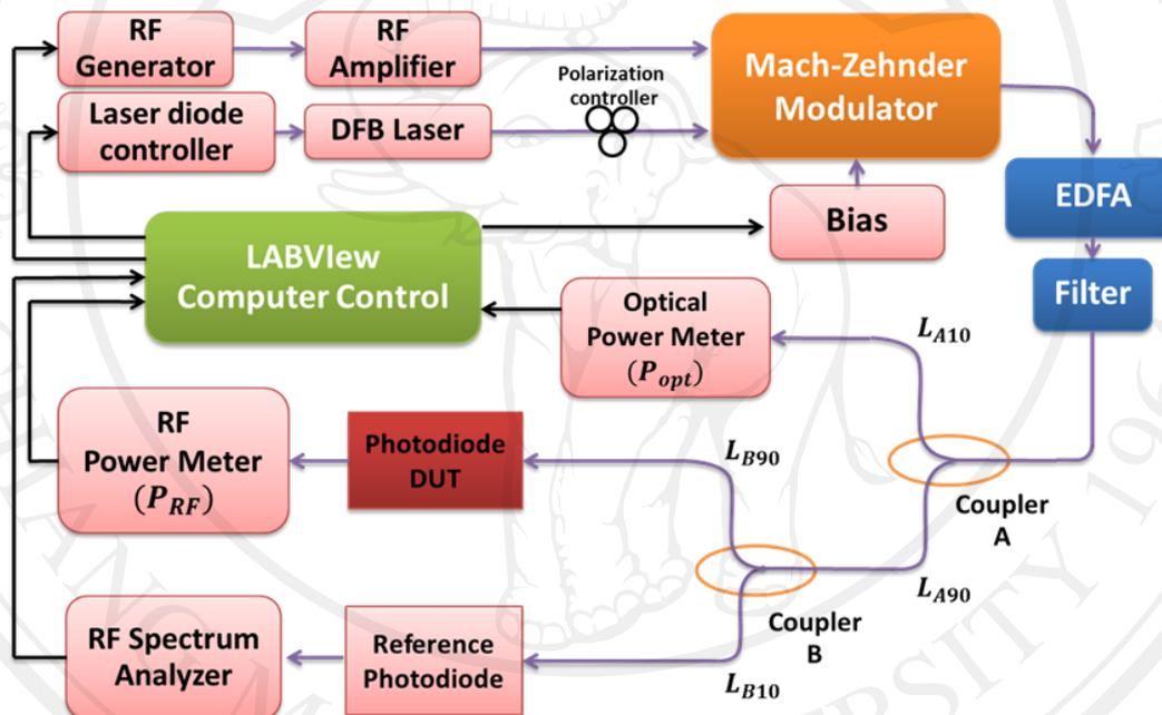
Figure 3.4 PD frequency response measurements using EDFA as a post-amp
