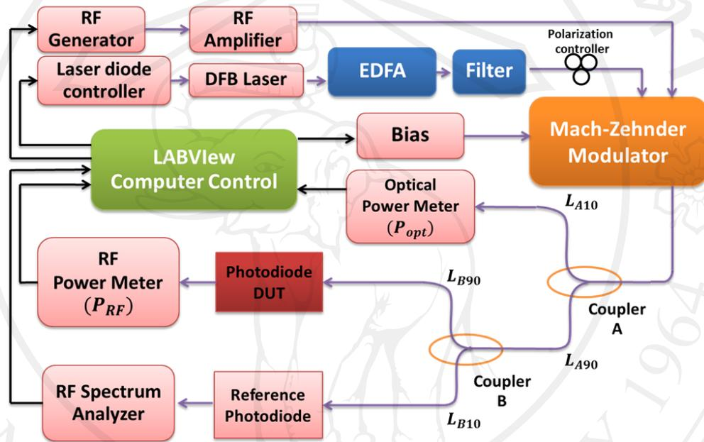
Figure 3.3 PD frequency response measurements using EDFA as a pre-amp
