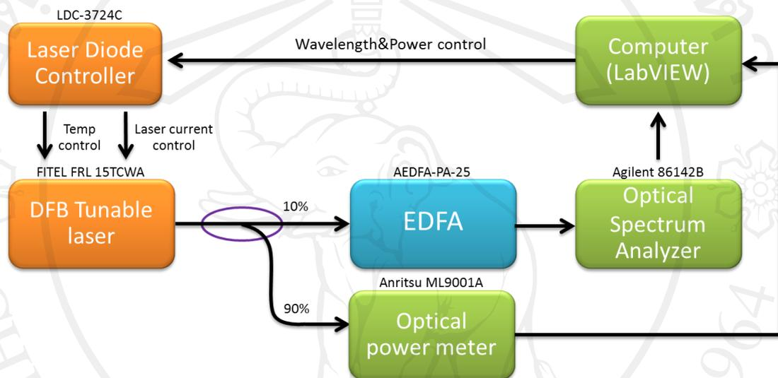
Figure 3.5 EDFA characterization measurement system
