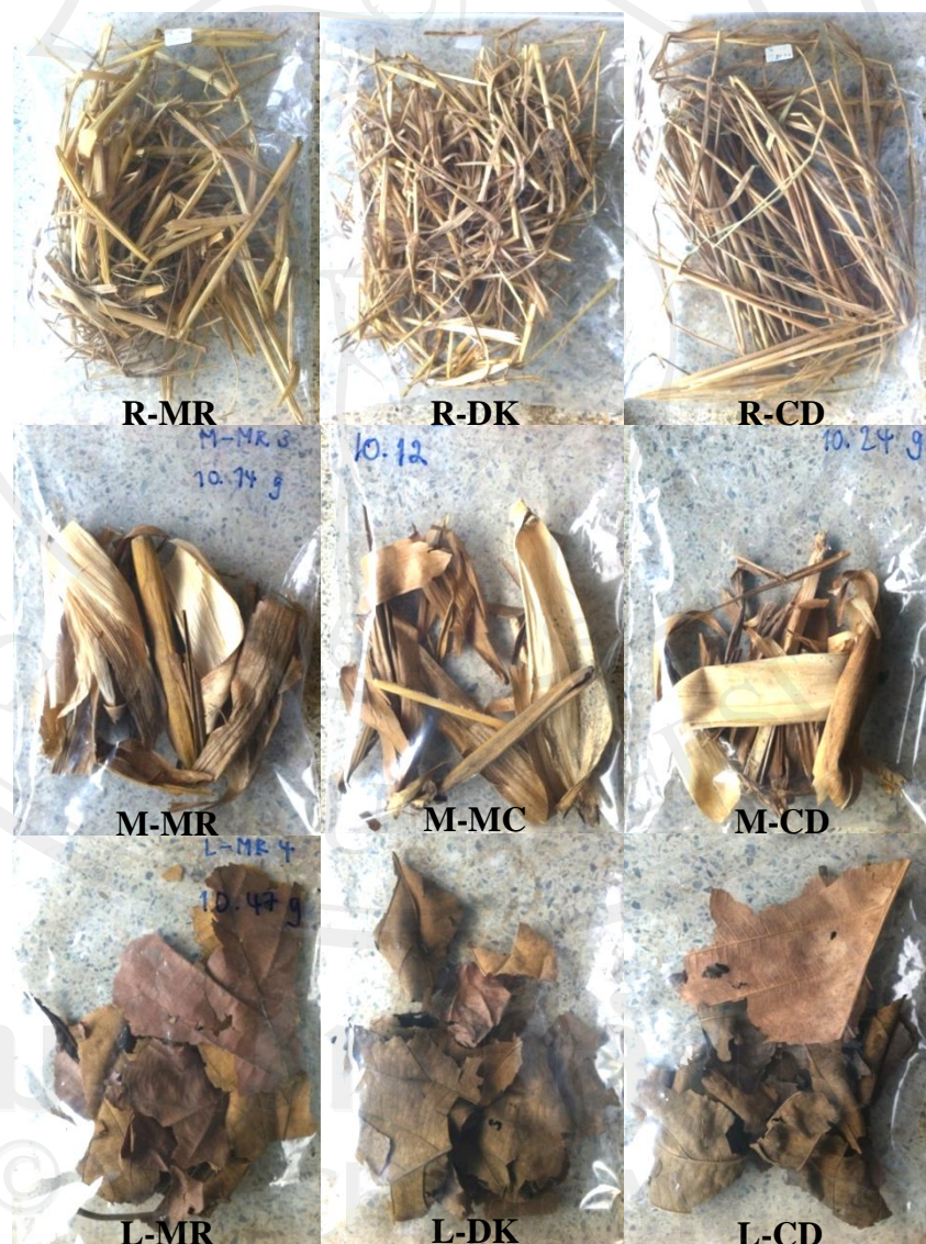
Figure 2.6 Biomass samples for burning experiment; rice straw (R), maize residue (M) and leaf litter (L)
