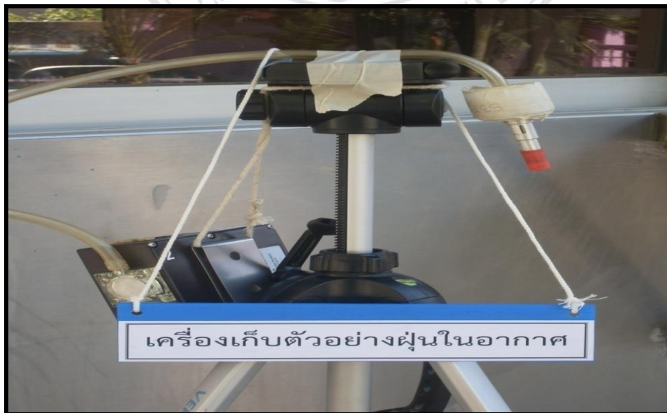
Figure 3.13 Personal air sampler, close-up, was used to monitor PM 10 level in the classroom
