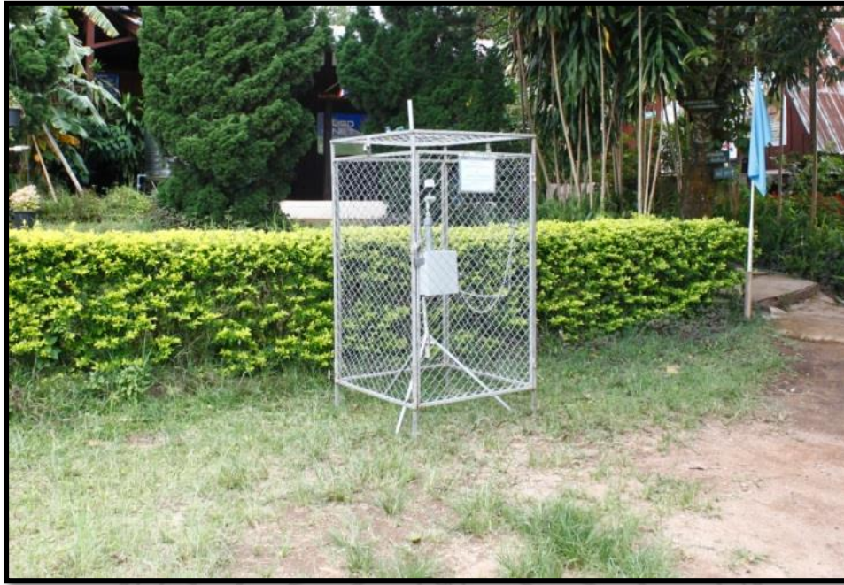
Figure 3.11 Portable air sampler used to monitored PM 10 level at the courtyard of SN school
