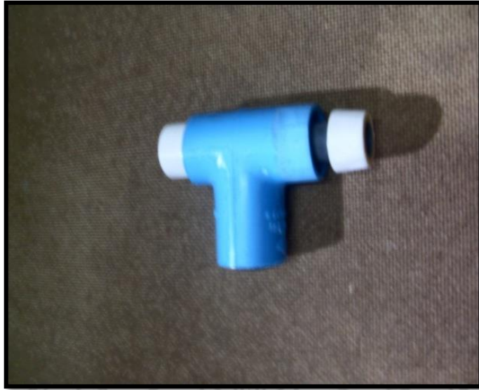
Figure 3.7 The second one-way valve
