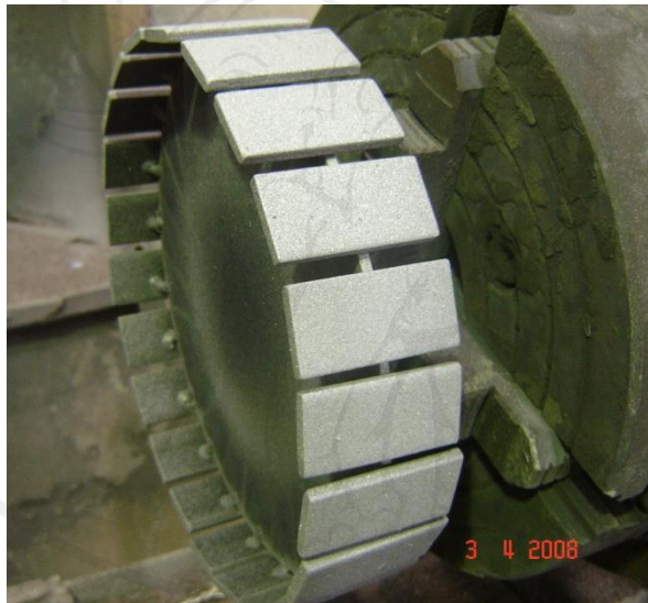
Figure 3.5 Installation of substrates on holder wheel and lathe machine.
