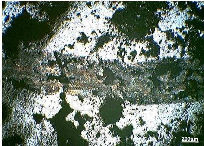
Figure 4.78 OM image shows wear track of WC-Cr-Fe coating at 100X magnification.
