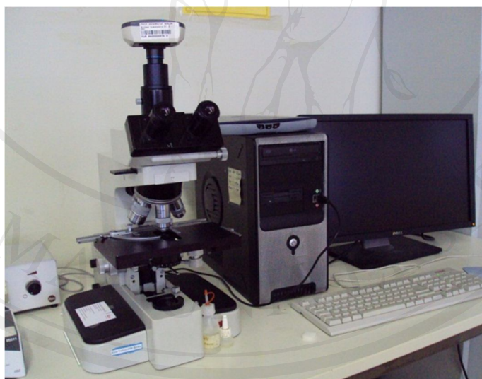
Figure 8 Light microscope (Leitz, Wetzlar, Germany) equipped with a CMEX-1 digital camera (Euromex microscopes, Arnheim, The Netherlands) connected to Image Focus software version 1.3.1.4. (Euromex microscopes, Arnheim, The Netherlands).
