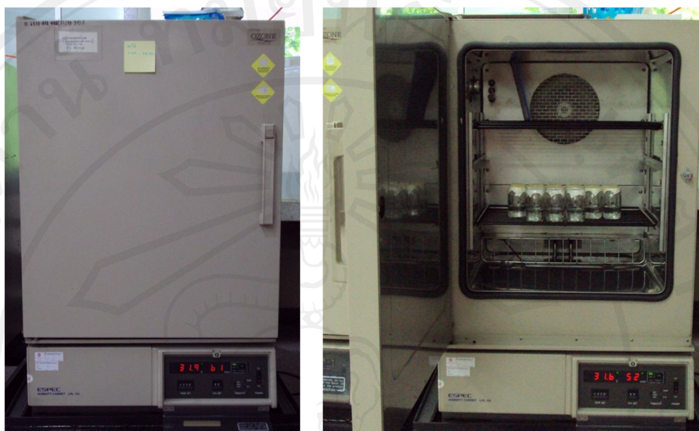
Figure 11 Occlusion test was performed in an oven which temperature is controlled at 32°C (skin temperature) and adjust to 60±5% relative humidity (%RH).
