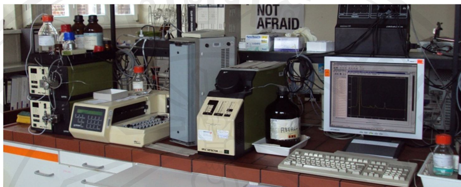
Figure 9 The HPLC system used consisted of an auto sampler model 360, a pump system model 420 and a UV visible detector model 430 (Kontron Instruments, Groß-Zimmern, Germany). This system was linked to a KromaSystem 2000 v. 1.83 data acquisition and process system, which also controlled the HPLC modules.
