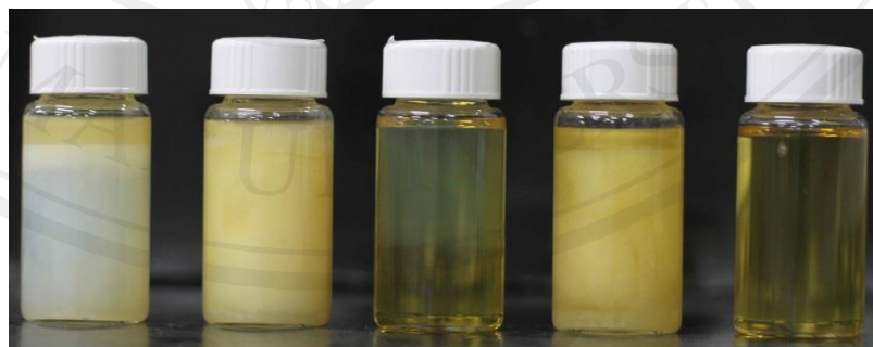
Figure 4.61 The outer appearance of sesame oil microemulsion systems without drug which were kept in various conditions. (HT = 45 °C, RT = Room temperature about 30 °C, LT = 4 °C, HCC = heating and cooling cycle)
