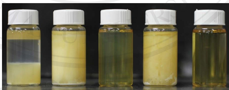
Figure 4.62 The outer appearance of sesame oil microemulsion systems with drug which were kept in various conditions. (HT = 45°C, RT = Room temperature about 30°C, LT = 4°C, HCC = heating and cooling cycle)
