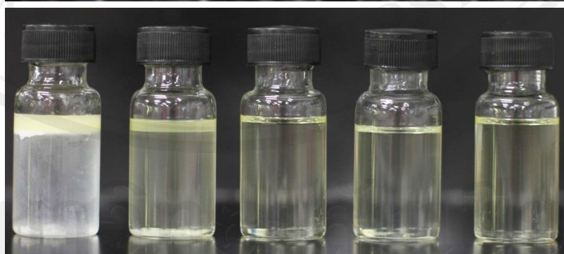
Figure 4.60 The outer appearance of lemongrass oil microemulsion systems with drug which were kept in various conditions. (HT = 45°C, RT = Room temperature about 30 C, LT = 4°C, HCC = heating and cooling cycle)
