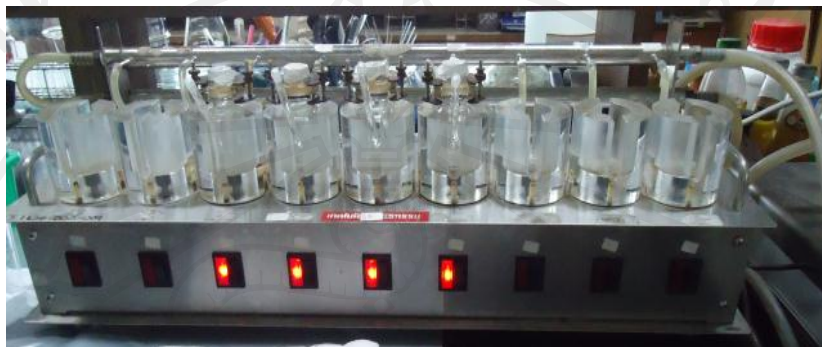
Figure 3.3 Modified Franz diffusion cell
