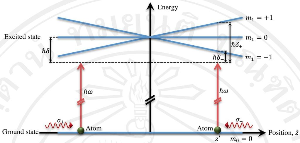
**Figure 2.3.** Cooling mechanism in one-dimensional MOT. The atomic ground state and first excited state are indicated by the total angular momentum of  $J = 0$  and  $J' = 1$  respectively. The excited state is split because of the Zeeman effect.
