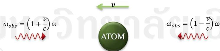
**Figure 2.2.** The Doppler effect in the laser cooling process in one dimension. The details are described in text.
