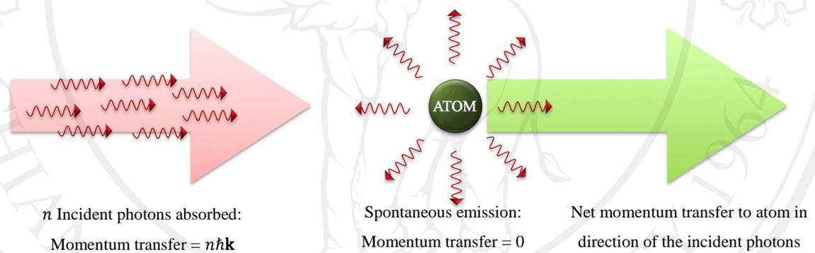
**Figure 2.1.** Momentum transfer in the laser cooling process. An atom at rest in laser beam absorbs a photon (represented by the small red arrow) in the incident laser beam, and then emits a photon spontaneously.
