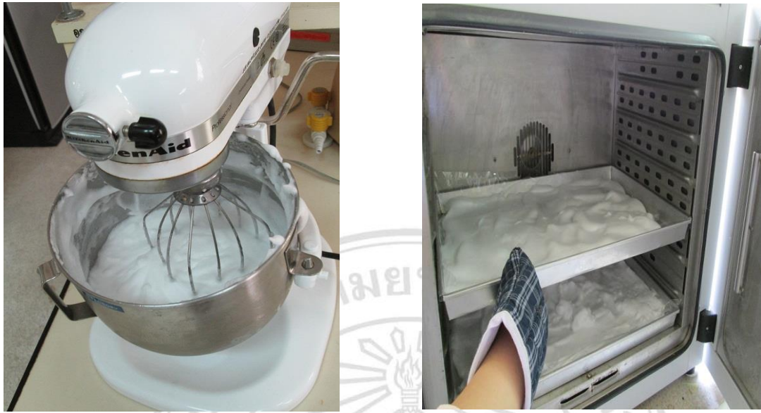
Figure A4 Salt preparation by foam-mat drying
