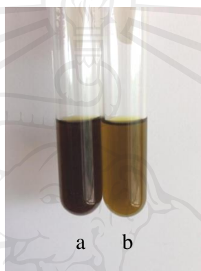
Figure 4.2 The sample solution from conventional technique (a), after treated with EC process (b)
