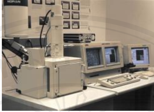
Figure 1.15 A typical SEM instrument, showing the electron column, sample chamber, EDS detector, electronics console, and visual display monitors [24]
