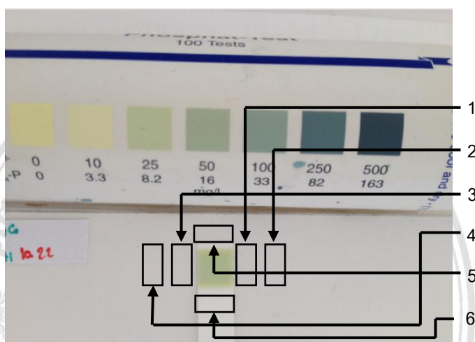
Figure 3.2 Image of the standard chart and the test strips taken in the white box and 6 measure points of background of the strips
