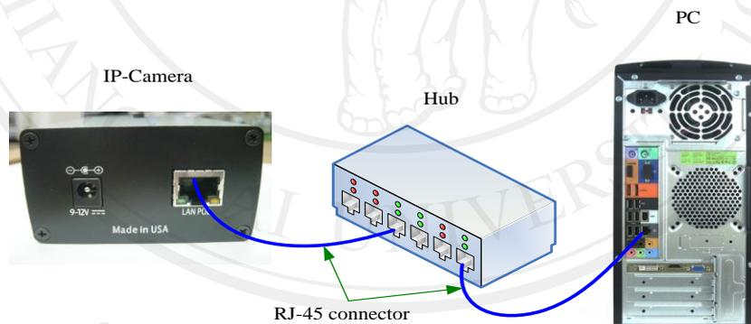
Figure A.1 Configuration of IP camera connections.
