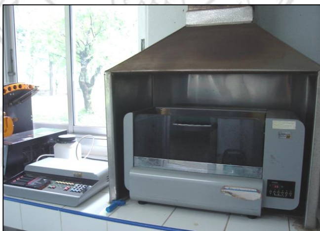
Figure 3.15 The furnace is used for XRF sample preparing
