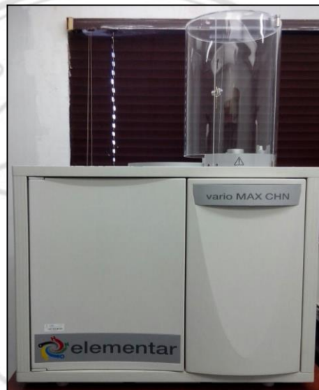
Figure 3.11 Elemental analyzer for carbon, hydrogen, and nitrogen in coal samples
