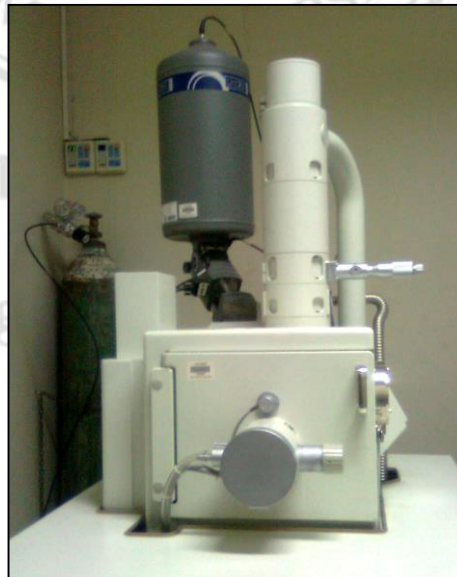
Figure 3.8 The scanning electron microscopy with dispersive x-ray spectroscopy
