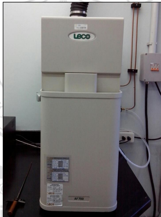
Figure 3.18 The ash fusibility determinator for measure the AFT
