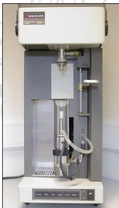
Figure 3.14 Thermogravimetric analyzer for nonisothermal isoconversional approach
