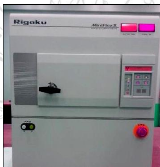
Figure 3.9 The X-ray diffraction analyzer
