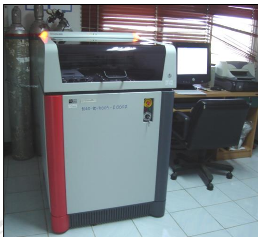
Figure 3.16 The XRF spectrometer for ash composition analysis
