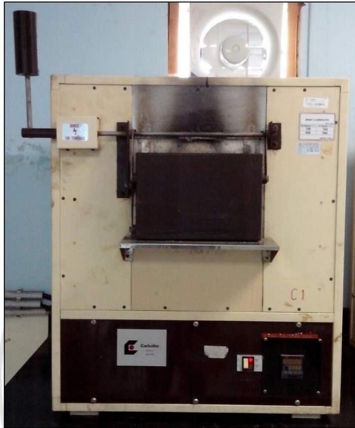
Figure 3.4 Carbolite furnace for prepare the ash samples
