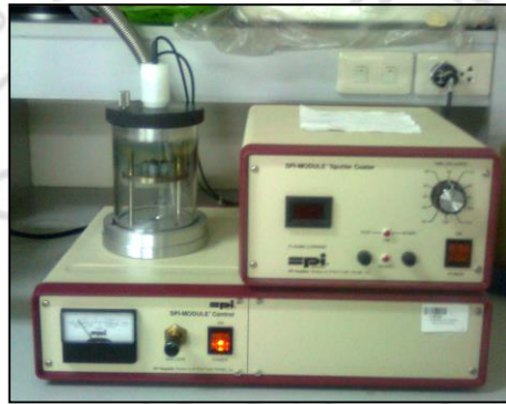
Figure 3.7 Gold sputter coater for SEM sample
