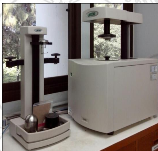
Figure 3.13 Bomb calorimeter for use to determine heating value of coal samples
