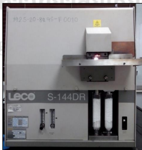
Figure 3.12 Sulfur analyzer for sulfur in coal samples
