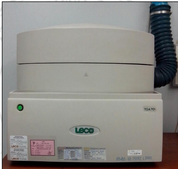
Figure 3.10 Thermogravimetric analyzer in Mae Moh power plant laboratory
