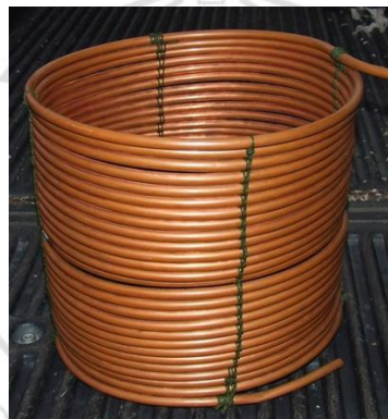
Figure B.20: Condenser coil constructed
