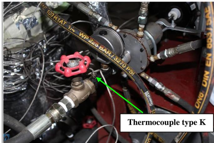
**Figure 3.12:** Thermocouple type K installation
