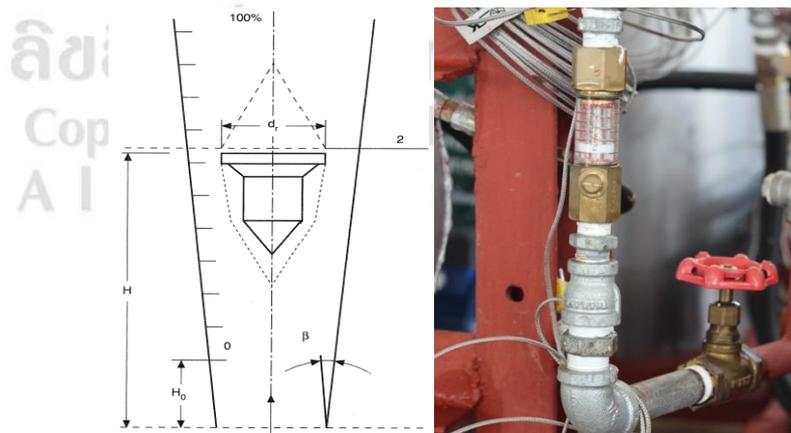
**Figure 3.17:** Rotameter measured for working fluid flow rate
