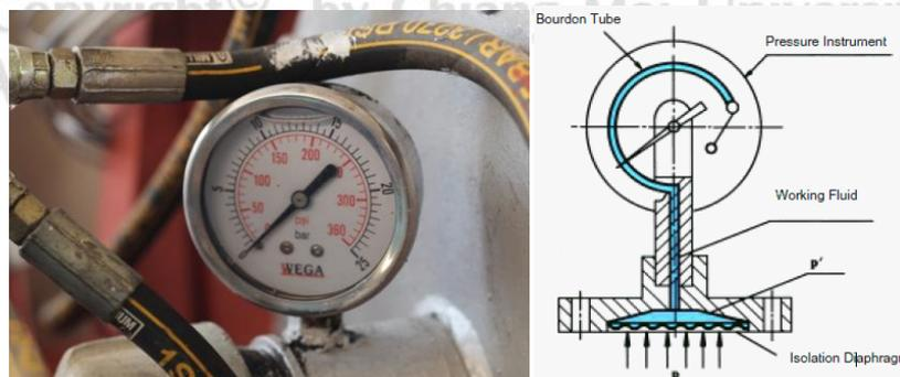
**Figure 3.14:** Pressure measurement by pressure gauge
