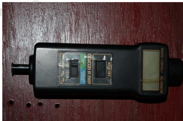
**Figure 3.18:** Tachometer measured for turbine shaft rotating
