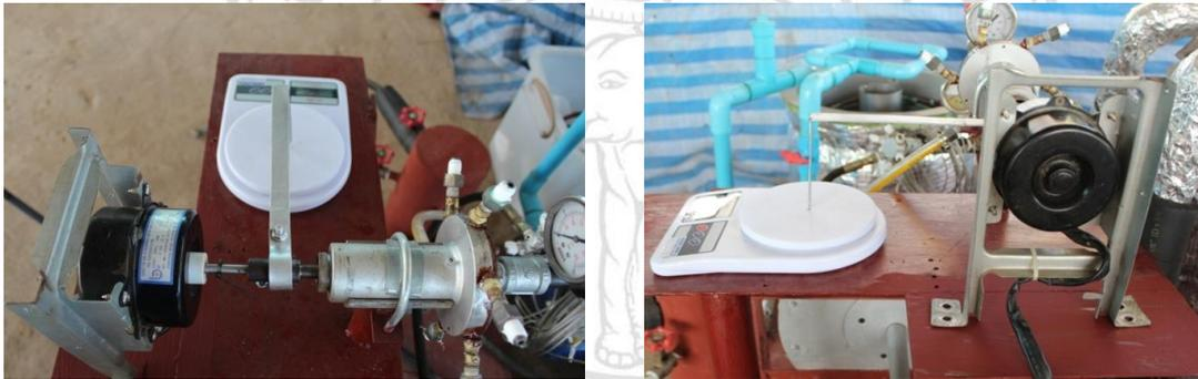
Figure 3.15: Prony brake installation for torque measurement
