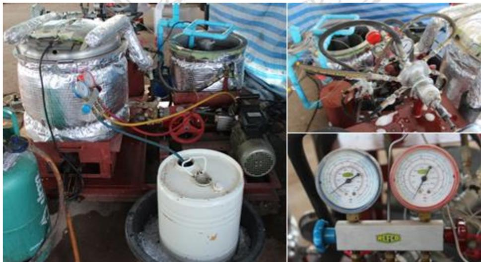
**Figure 3.11:** Working fluid leak checked and charging
