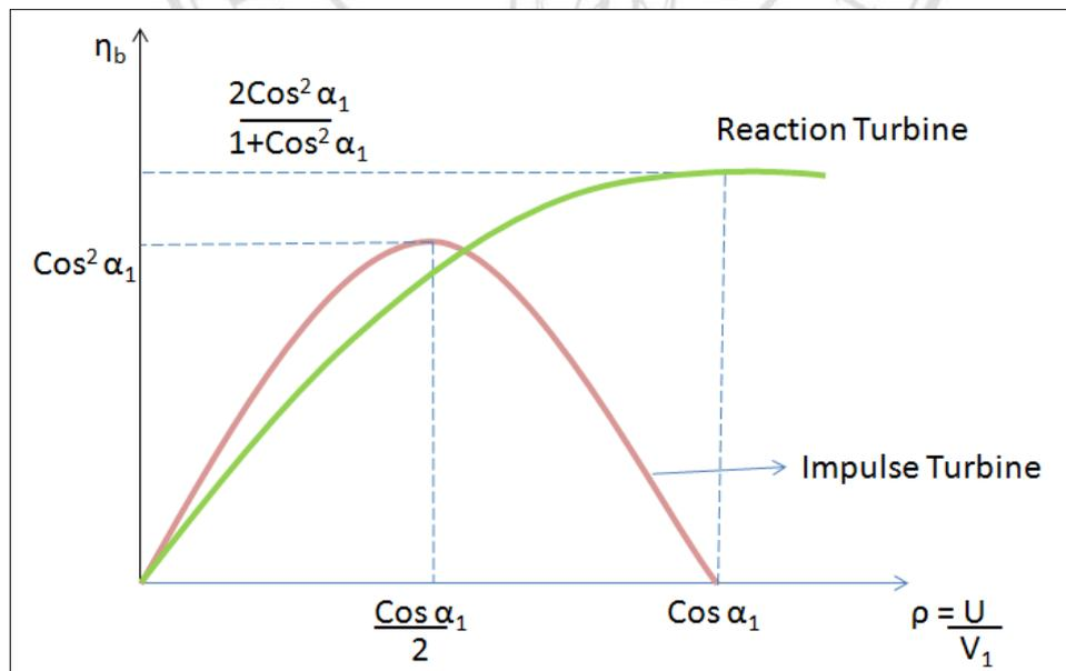
**Figure 3.2:** Characteristic curves for efficiency of turbines
