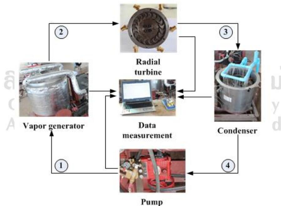
**Figure 3.1 (a):** ORC test rig diagram
