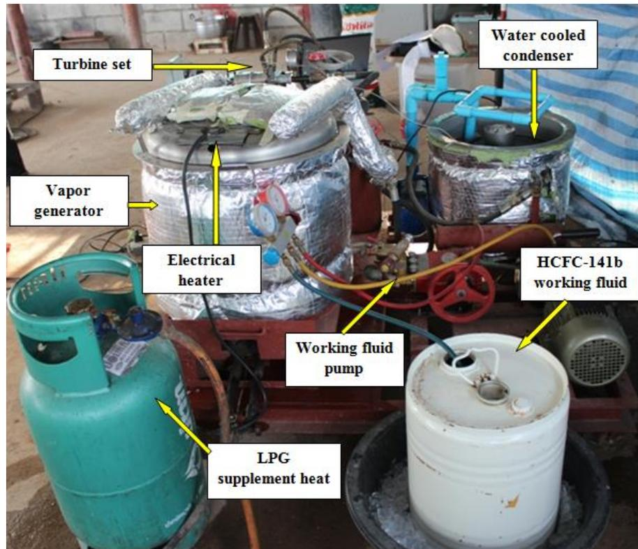
**Figure 3.1 (b):** ORC test rig
