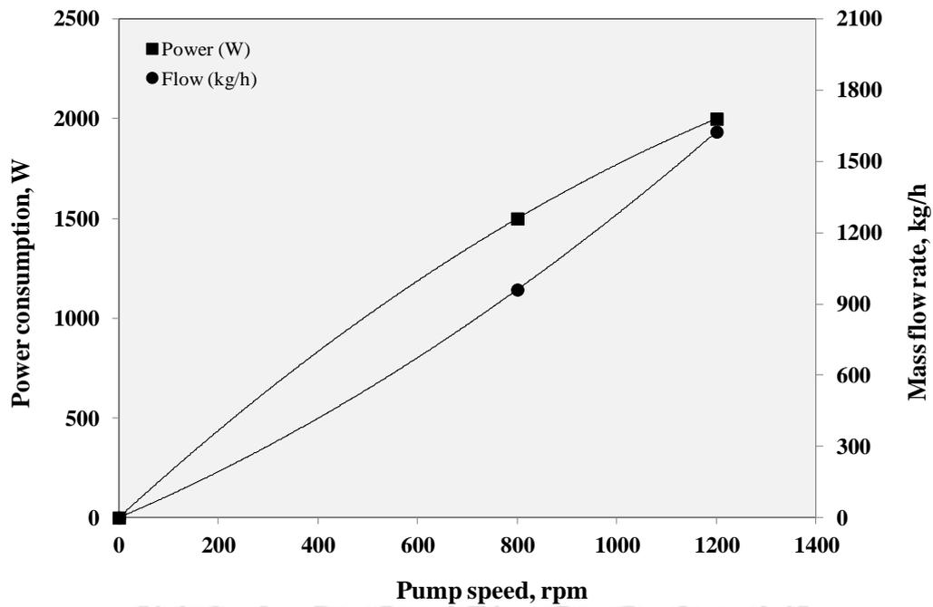
**Figure 3.9:** Characteristic of working fluid pump.
