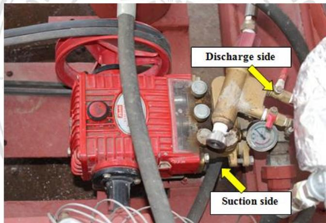
**Figure 3.8:** Working fluid pump installation
