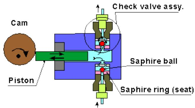
**Figure 3.7:** Schematic of reciprocating piston pump
