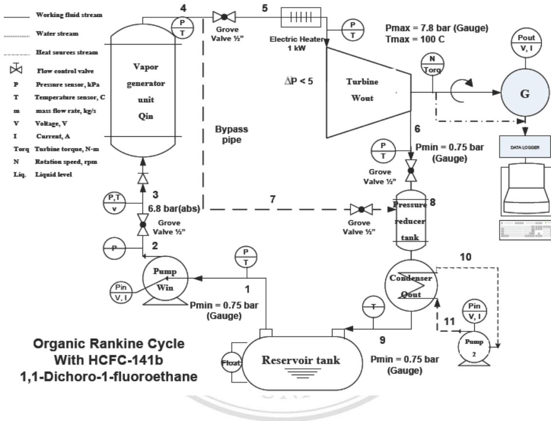
**Figure 3.19:** Schematic diagrams of experimental apparatus components
