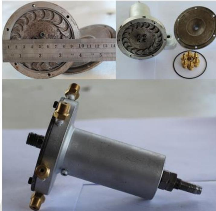
**Figure 3.4:** Assembly of impulse radial turbine set
