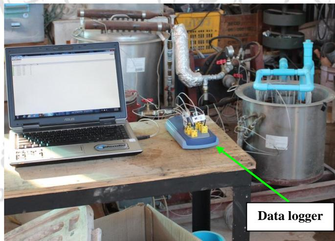
**Figure 3.13:** Temperature data logger measured
