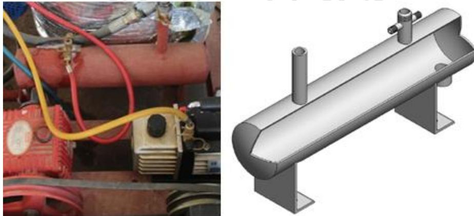
**Figure 3.10:** Receiver tank design and installation
