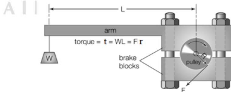
Figure 3.16: Schematic diagram of torque measurement
