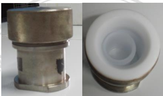
Figure 3.3 Double layer Teflon digestion vessel (Qiuquan et al. 2003)
