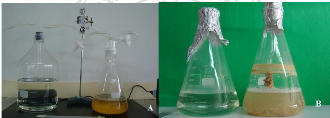
Figure 22 Culture in 1 liter of modified bubble column bioreactor.
