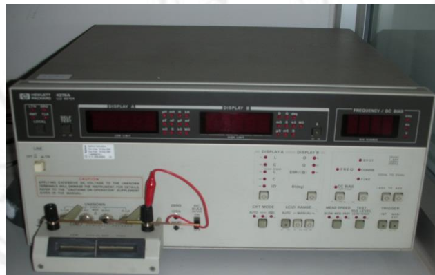
Figure 3.27 The dielectric properties measurement at room temperature.
