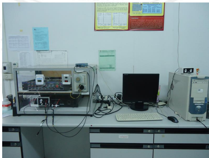
Figure 3.30 Ferroelectric hysteresis loop measurement.
