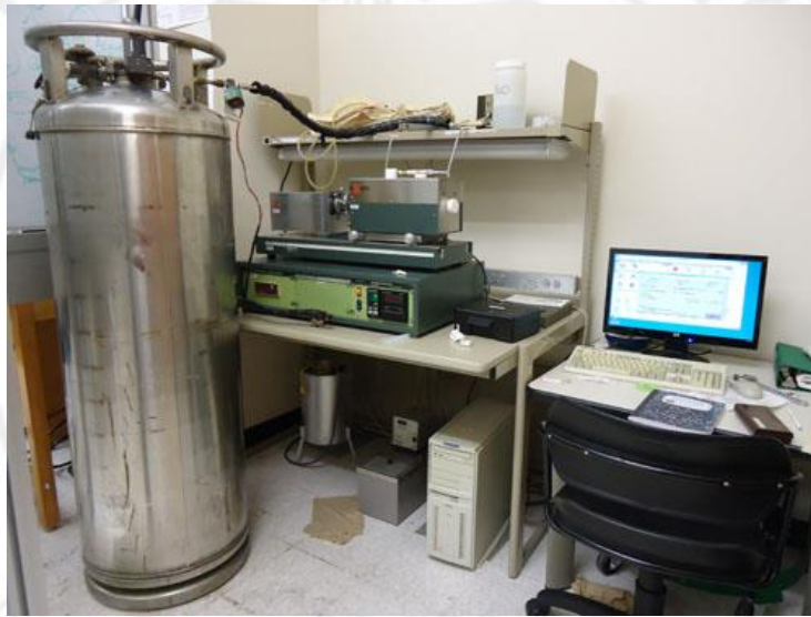
Figure 3.26 The thermal expansion measurement.
