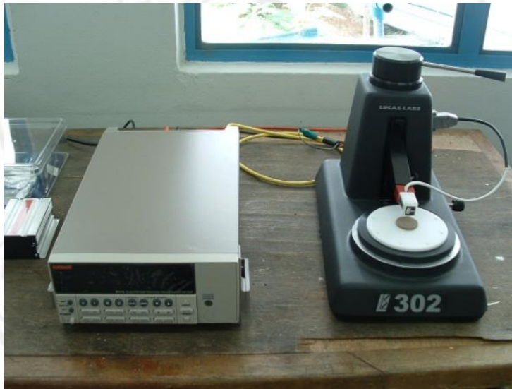
Figure 3.29 The resistivity and conductivity measurements.
