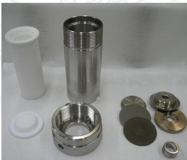
Figure 1.11 General purpose autoclave popularly used for hydrothermal synthesis [63].
