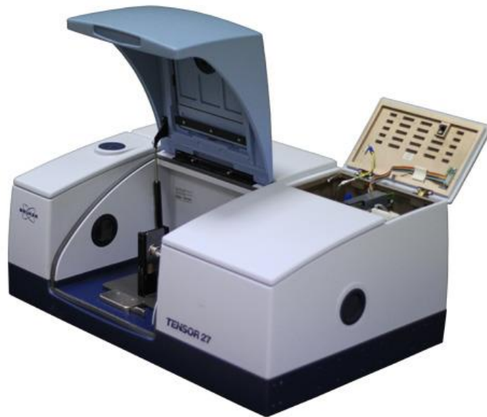
Figure 3.6 Fourier transform infrared spectroscope
