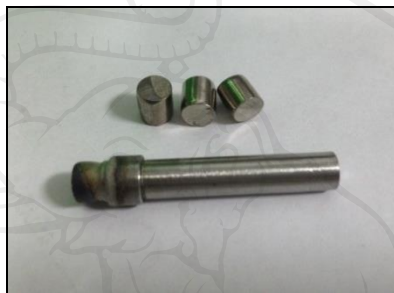
Figure 3.1 Small pure titanium rod is attached to the end of stainless steel rod.
