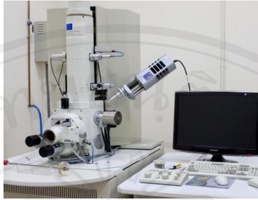
Figure 3.11 The JEOL® JSM 6335F is being used for analyzing the film by both SEM and EDS techniques in this study.
