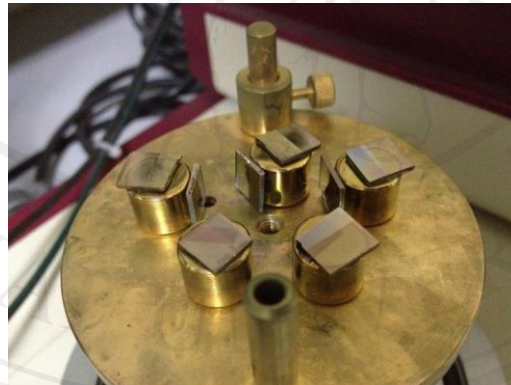
Figure 3.10 Gold-coated TiO 2 -deposited substrates attached on top and side of SEM's stubs.
