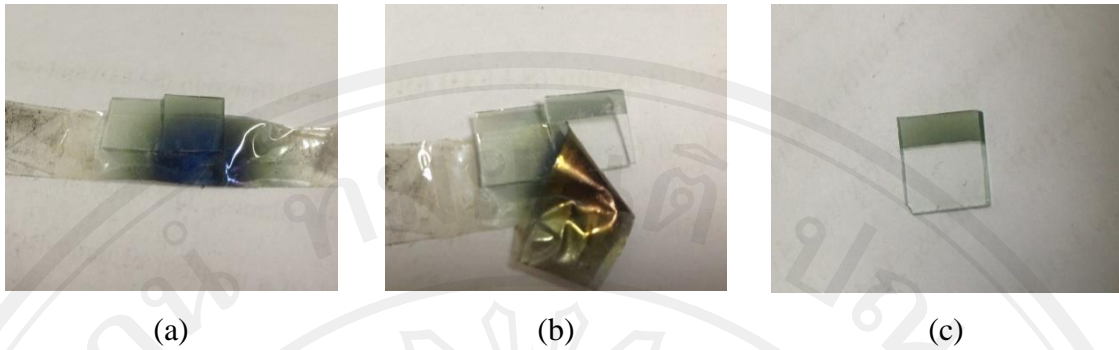
Figure 3.8 The \text{TiO}_2 post-deposited substrates (a) partly transparent tape pasted, (b) after removing of the tape, it is ready to be analyzed its thickness by AFM (c).
