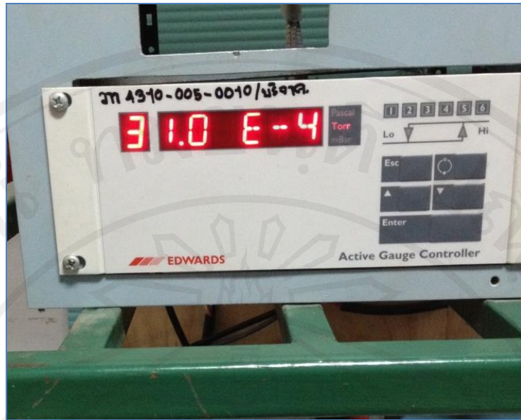
Figure 3.4 Active gauge controller is being used to measure the deposition chamber's pressure lower than 2 \times 10^{-2} torr.
