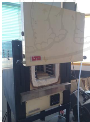
Figure 3.9 The LTD® annealing furnace is being used for annealing \text{TiO}_2 film.
