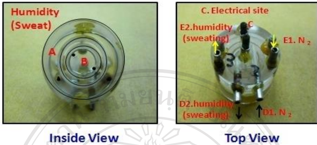
Figure 3.5 Hygrometer-ventilated capsule method was used to determined sweat gland function.
