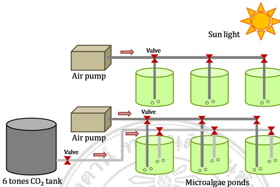
Figure 6.2 Schematic diagram of microalgal cultivation using pure CO<sub>2</sub> in an outdoor open system
