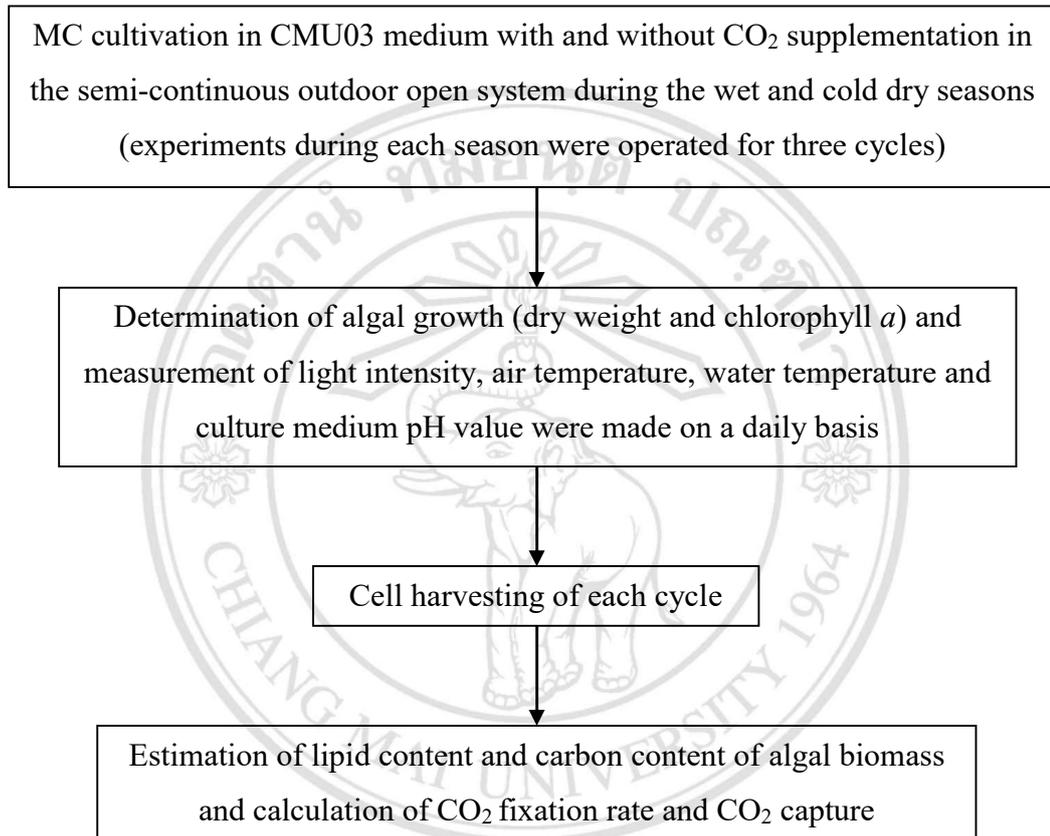
Figure 6.1 Flowchart diagram of microalgal cultivation using pure CO<sub>2</sub> in an outdoor open system
