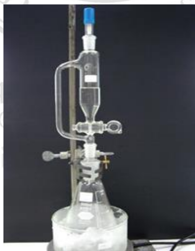
Figure 5.2 Apparatus used for PCL purification by re-precipitation from solution.
