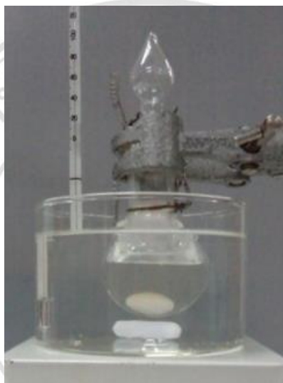
Figure 5.1 Apparatus used in the ring-opening bulk polymerisation of \epsilon -CL.
