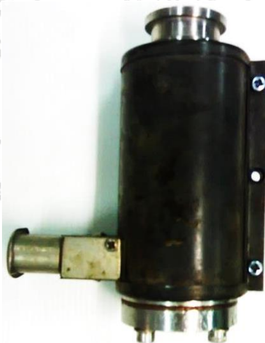
Figure 7.3 The assembled cylinder used for making a copolymer rod.
