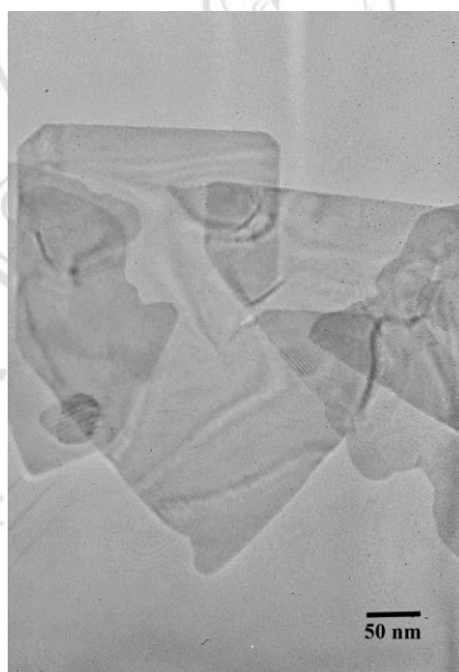
Figure 3.6 TEM images of CMC-AgInS 2 QDs synthesized by hydrothermal method (sample 6).
