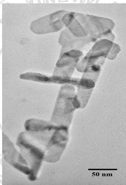
Figure 3.4 TEM images of CMC-AgInS 2 QDs synthesized by hydrothermal method (sample 4).
