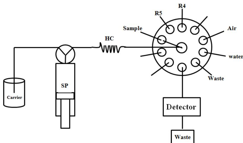
**Figure 2.4** Sequential injection (SI) colorimetric system diagram for phosphate determination. SP = 2.5 mL barrel syringe pump, HC = holding coil, R4 = 10.0 g L<sup>-1</sup> ammonium molybdate, R5 = 2.5% w/v ascorbic acid
