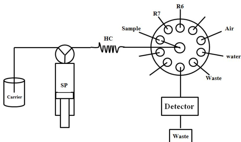
**Figure 2.5** Sequential injection (SI) colorimetric system diagram for ammonium determination. SP = 2.5 mL barrel syringe pump, HC = holding coil, R6 = 0.5% w/v sodium hypochlorite and R7 = 0.4 mol L<sup>-1</sup> sodium salicylate
