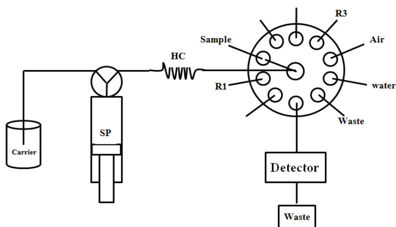
**Figure 2.3** Sequential injection (SI) colorimetric system diagram for manganese determination. SP = 2.5 mL barrel syringe pump, HC = holding coil, R1 = 5.0% hydroxylamine, R3 = 0.6 mol L<sup>-1</sup> formaldoxime
