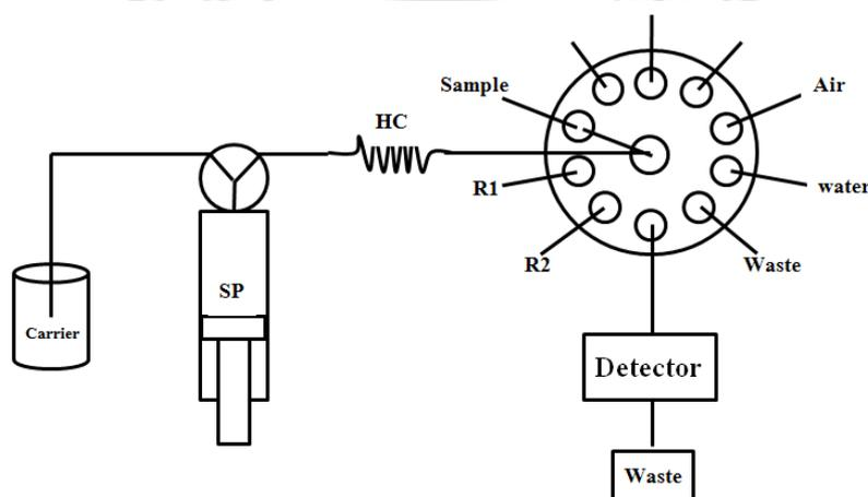
**Figure 2.2** Sequential injection (SI) colorimetric system diagram for iron determination. SP = 2.5 mL barrel syringe pump, HC = holding coil, R1 = 5.0% hydroxylamine, R2 = 0.5% w/v 1,10-phenanthroline
